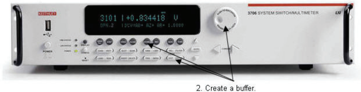
Figure 16: Create a buffer to save readings on a USB flash drive
