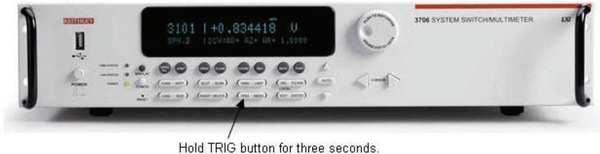
Figure 12: Instrument TRIG button
