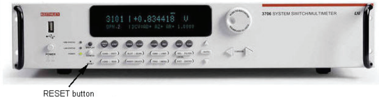
Figure 5: LAN reset button
