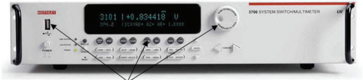
Figure 18: Store the buffer on a USB flash drive
