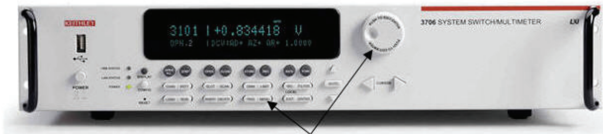
Figure 11: Instrument factory reset controls
