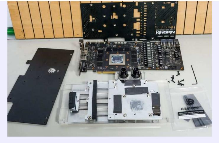
We will use native EVGA KPE backplate, to keep access for switches and LEDs. In such case stock screws should be used to mount block, as Bitspower screws are made longer to fit with thicker BP backplate.
