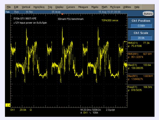
All results were captured with GPU cooled to -100°C, using Tektronix TDS5034B scope and TCPA303 current probe.
