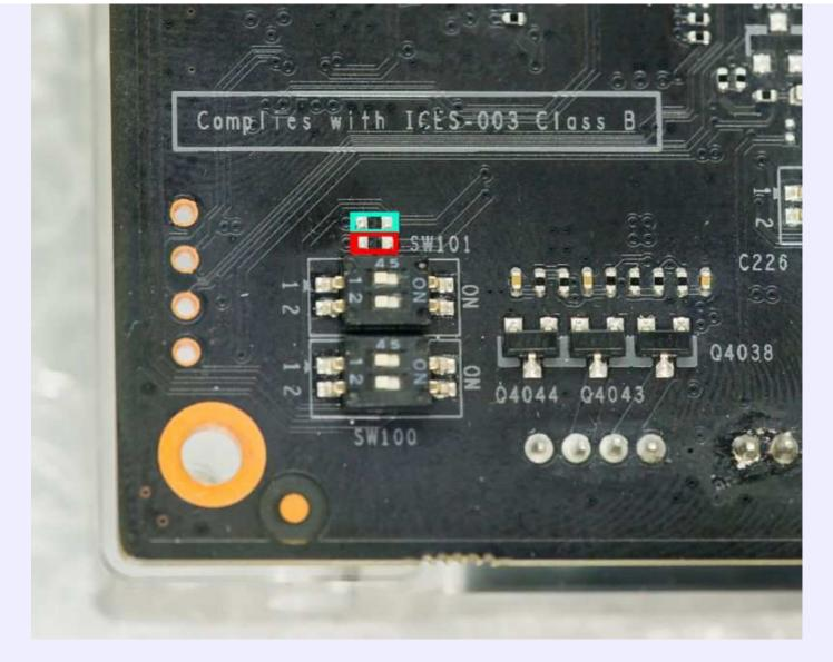
Shorted pads in cyan box enable memory voltage trimmer, while red pads short enable GPU voltage trimmer.
