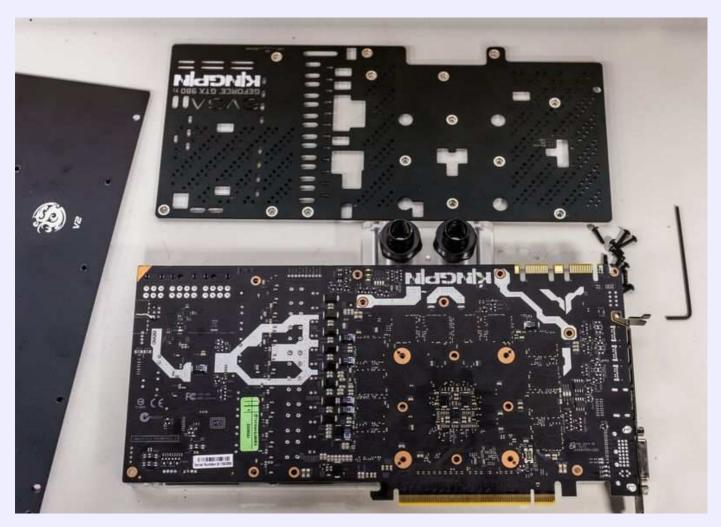
Installed block, front & back side
