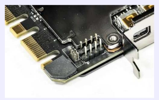
You have access to this port with both stock fansink operation and watercooling/LN2. Connect UART cable to VGA's serial port like this photo below. It could be little tricky to get cable between fansink cover, so use twizzers to fix cable in position.
