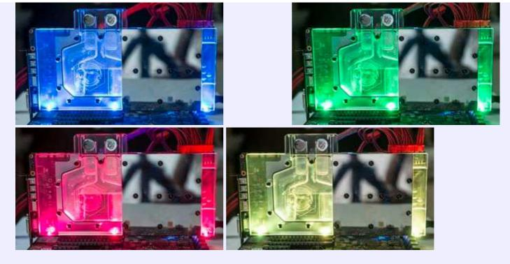
You can connect each LED to separate port (connectors J17,J18,J19) to control LEDs individually. Only your imagination is a limit for color scheme.
