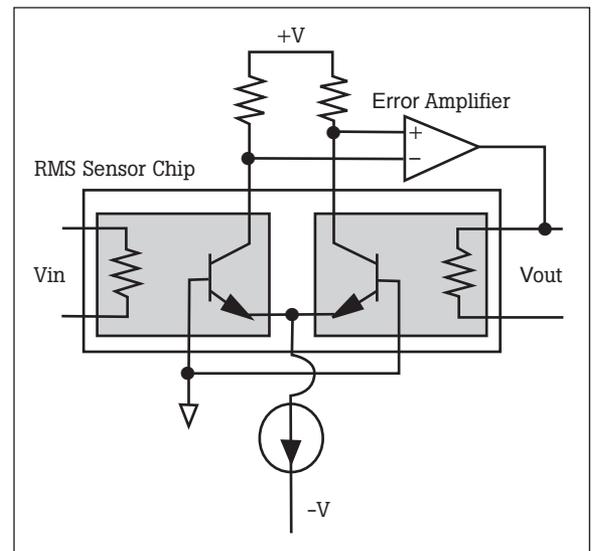
Figure 1. Simplified RMS sensor circuit.
