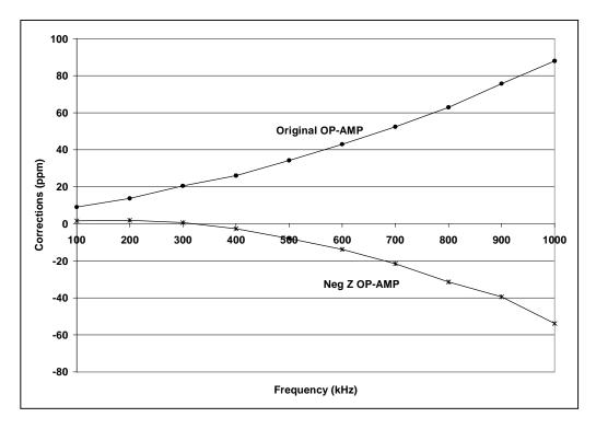
Figure 4. 792A Corrections with Different Vendor's OP-AMPs, 600 mV on 700 mV Range
