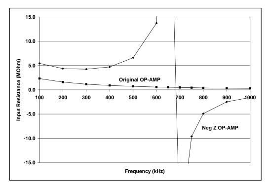
Figure 5. 792A Input Resistance with Different Vendor's OP-AMPs, 20 mV on 22 mV Range
