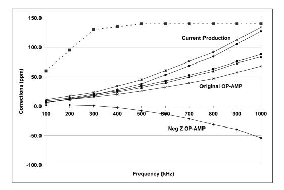
Figure 7. 792A Corrections for a Sample of Units, 600 mV on 700 mV Range
