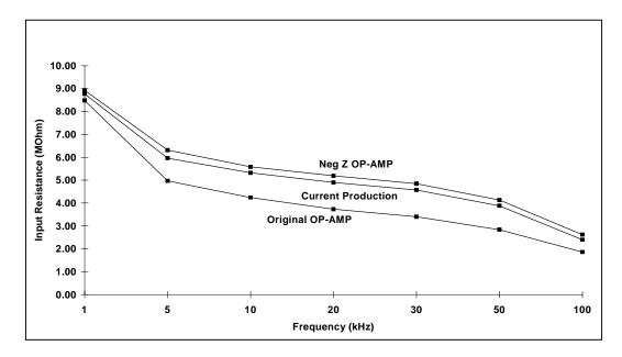
Figure 12. 792A Input Resistance, 1 kHz to 100 kHz, 200 mV on 220 mV Range
