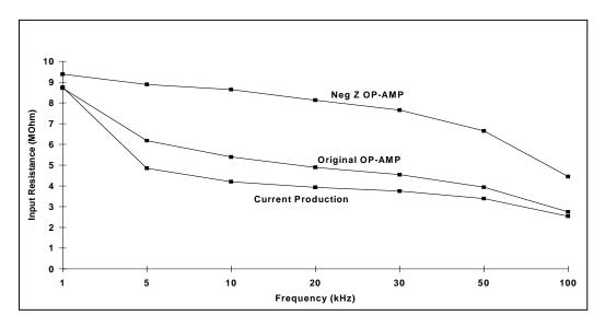
Figure 11. 792A Input Resistance, 1 kHz to 100 kHz, 600 mV on 700 mV Range
