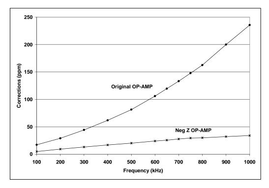
Figure 6. Corrections with Different Vendor's OP-AMPs, 20 mV on 22 mV Range
