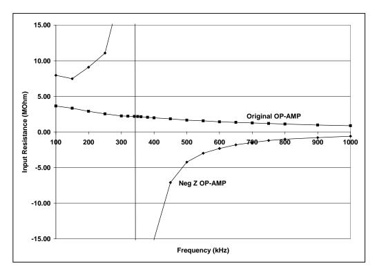
Figure 3. 792A Input Resistance with Different Vendor's OP-AMPs, 600 mV on 700 mV Range
