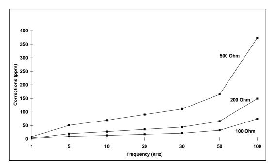
Figure 13. 792A Corrections for Loading of Current Shunts, 200 mV on 220 mV Range
