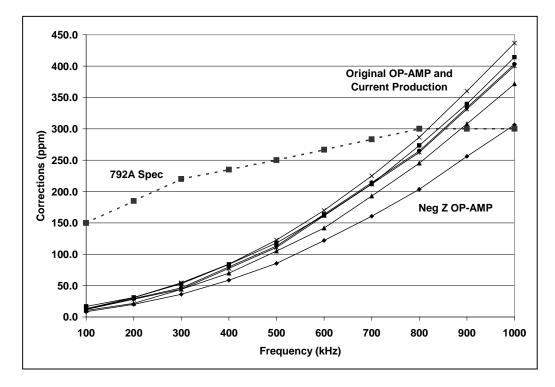
Figure 8. 792A Corrections for a Sample of Units, 200 mV on 220 mV Range
