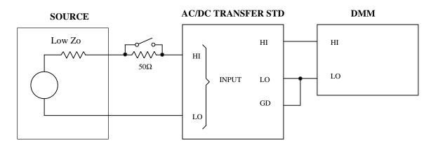
Figure 10. Method for Measuring Loading
