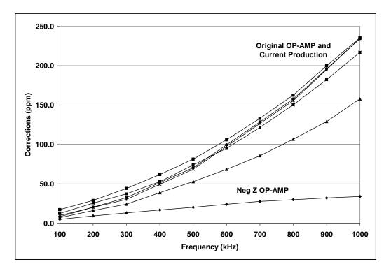
Figure 9. 792A Corrections for a Sample of Units, 20 mV on 22 mV Range
