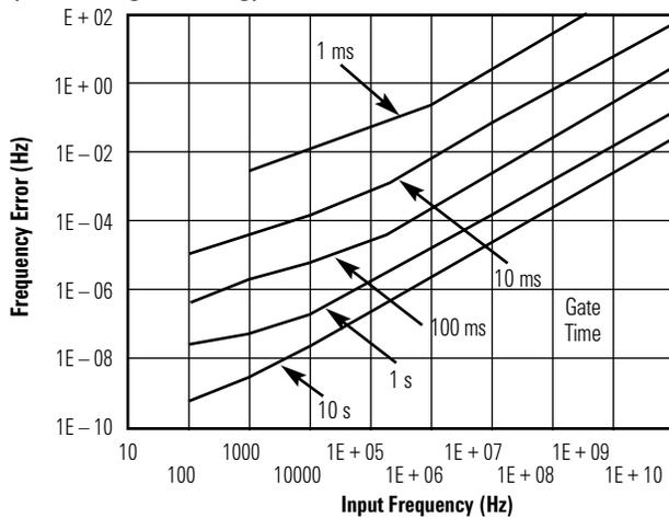
**Graph 6: Trigger Level Timing Error
