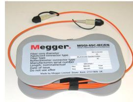
These contain approximately 100 meters of fiber with an SC connector to the XC-8513. Inside the box there is the appropriate mandrel configuration to aid equilibrium mode distribution. The XC-8513 is a duplex instrument and will automatically switch between the A and B measurement ports. To take advantage of this feature the two ports need to be combined into a normal duplex cable using the Duplex versions of the Mode Conditioning Patchcord box.
