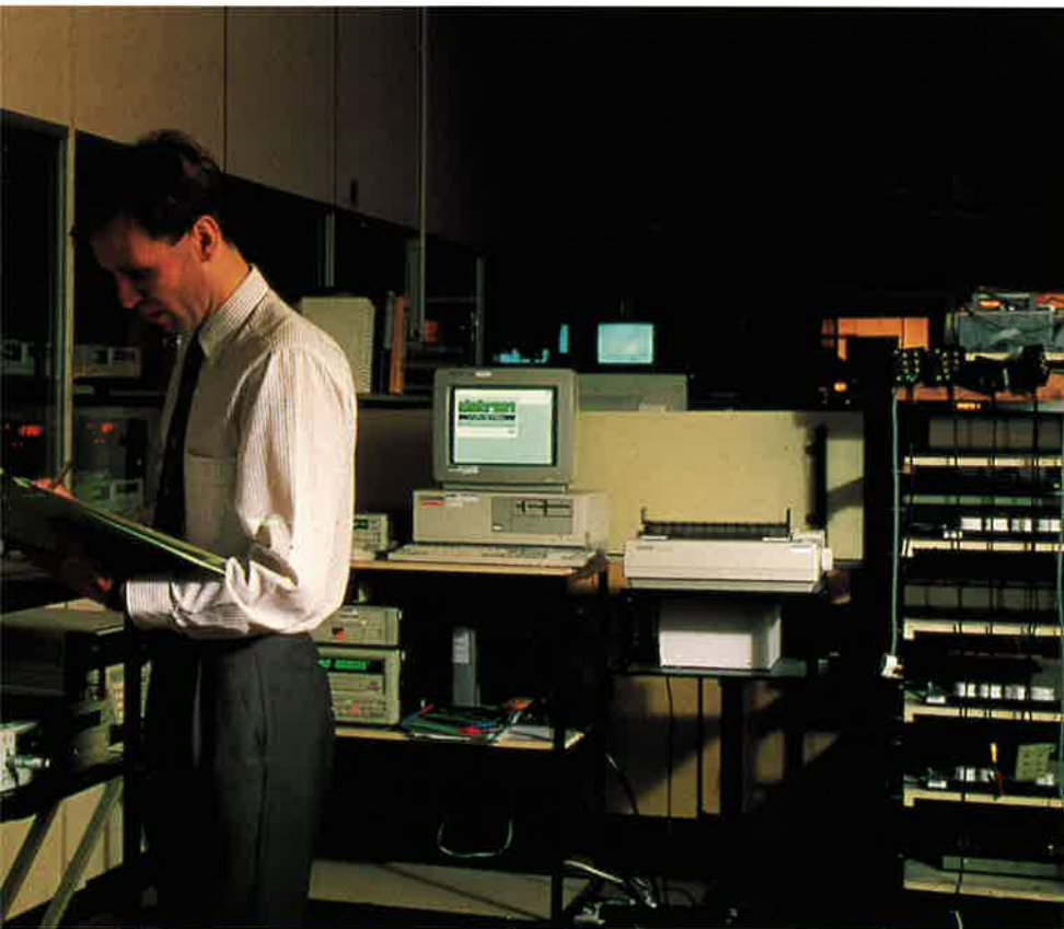
Multifunction calibrators are prepared for overnight calibration as part of the Wavetek Datron Division manufacturing process.
