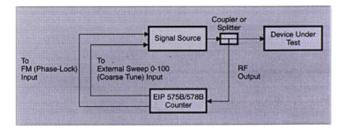
Only three connections are required to coarse tune and then phase lock an electrically tunable source
