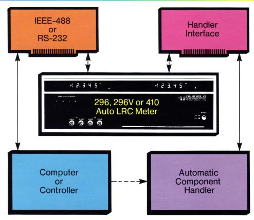
You can also program in multiband tolerance sorting. For reactance or loss. In absolute or percent deviation. With up to 10 limits, giving 9 accept bands and one reject band for highs and lows. In addition, a single maximum limit can be programmed for a second loss reject parameter. Bridge settling time is also under program control, from 25ms to 1.0 second, in 10ms increments.
