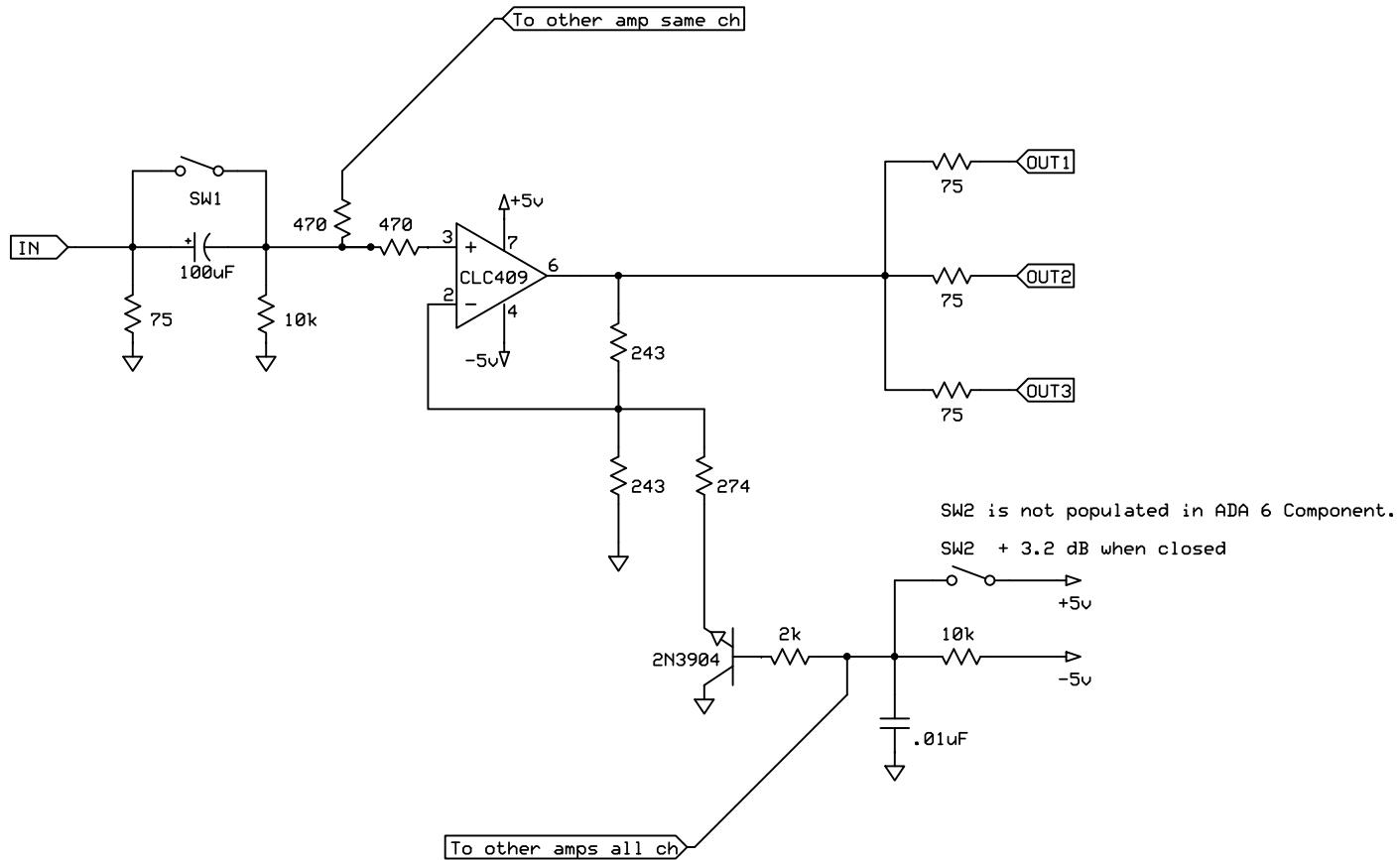
Schematic represents 1/6 of unmodified ADA 6 Component. Power supply not shown.
