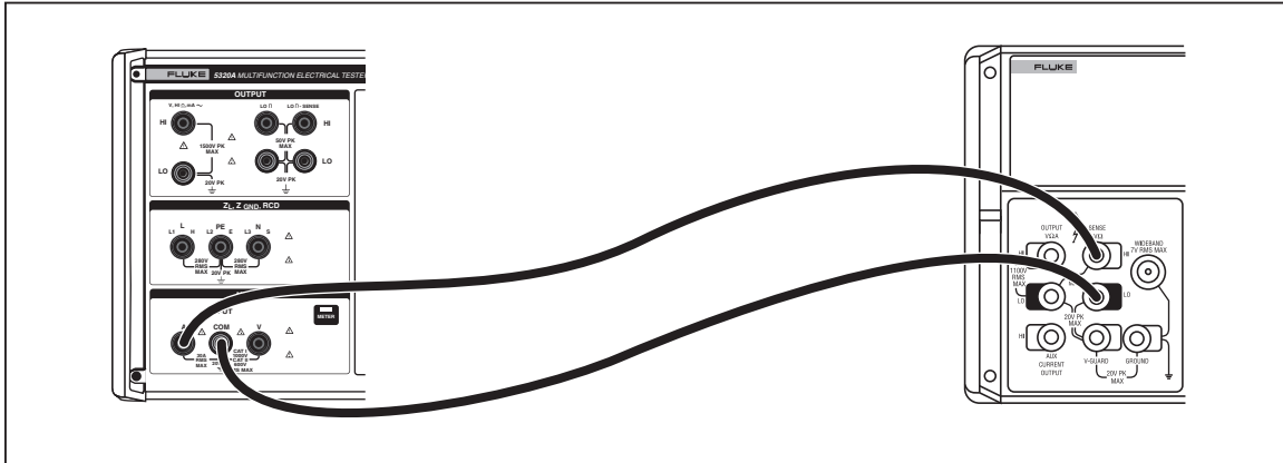
Figure 3-15. DC Multimeter Current Calibration Connections
