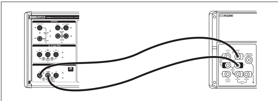
Figure 3-17. AC Multimeter Current Calibration Connections
