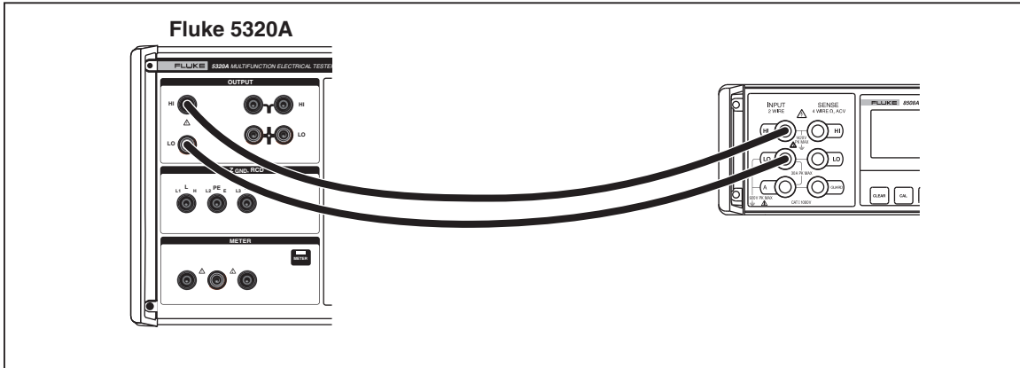
Figure 3-13. AC Voltage Calibrator Calibration Connections
