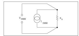
Figure 6. The DMM supplies a known current across  $R_{\rm x}$  the unknown resistance, and measures the resulting voltage.
