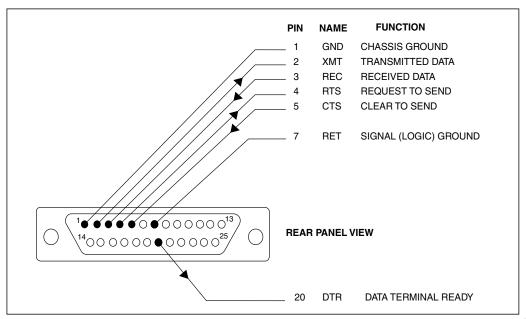
Figure 7-1. RS-232 Connector Pinout
