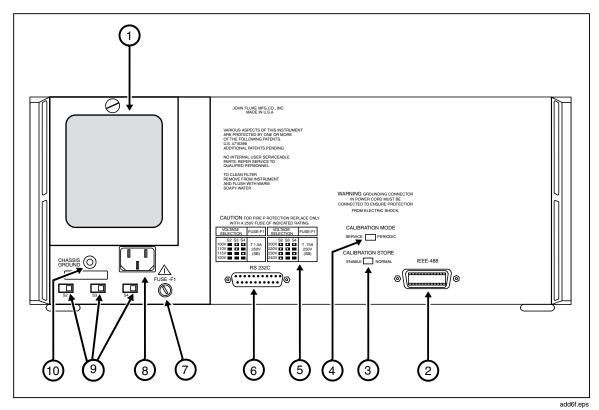
Figure 3-2. Accessing the Air Filter
