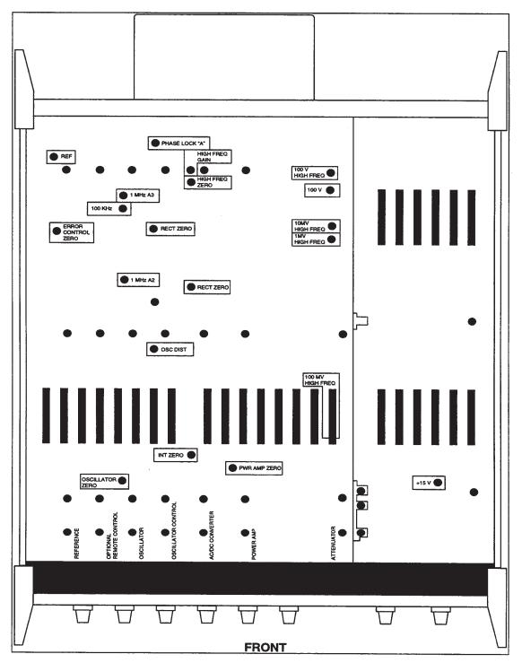
Figure F-6. Labeled Adjustment Ports
