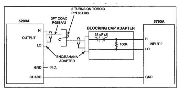
Figure F-5. 1 mV Output Accuracy Equipment Configuration
