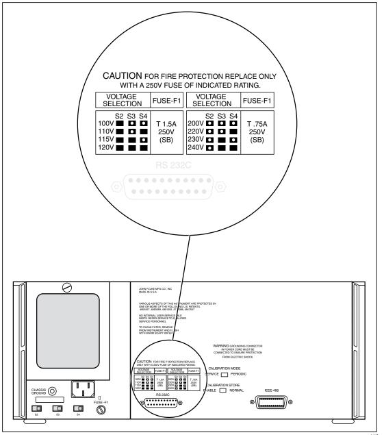
Figure 2-3. Line Power Label and Switch Location
