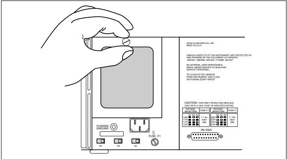
Figure 8-2. Accessing the Air Filter
