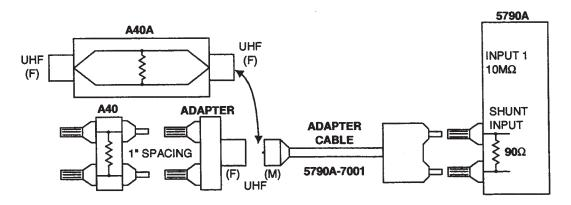
Figure 4-3. Measuring Relative Current Using 5790A-7001
