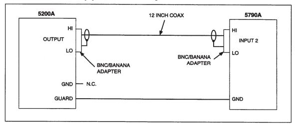
Figure F-3. 100 mV Output Accuracy Equipment Configuration
