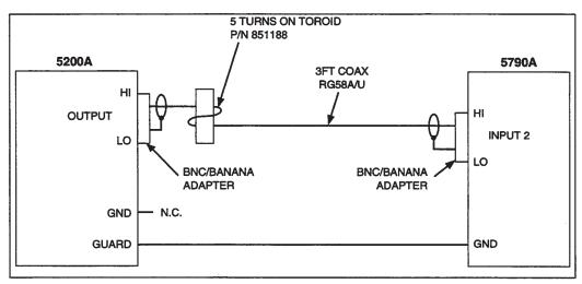
Figure F-4. 10 mV Output Accuracy Equipment Configuration
