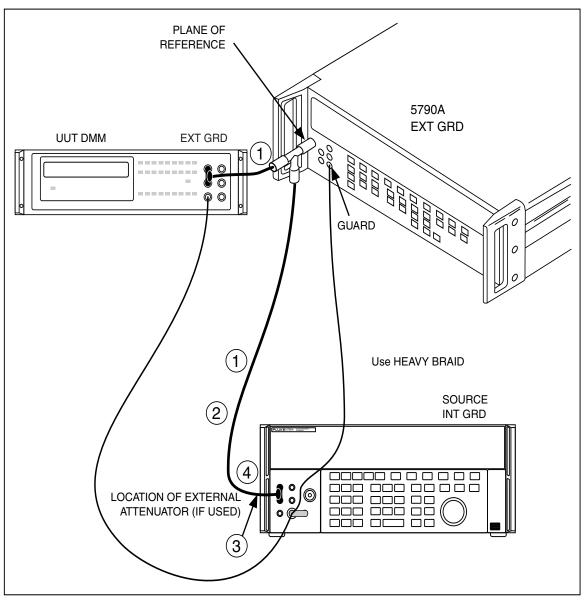
Figure 4-1. Recommended Test Lead Connections to Test a Voltmeter
