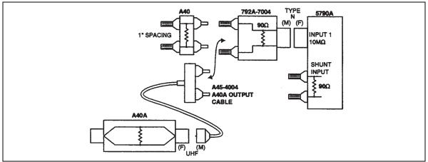
Figure 4-4. Measuring Relative Current Using 792A-7004
