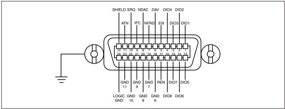
Figure 5-5. IEEE-488 connector pinout (Rear Panel View)
