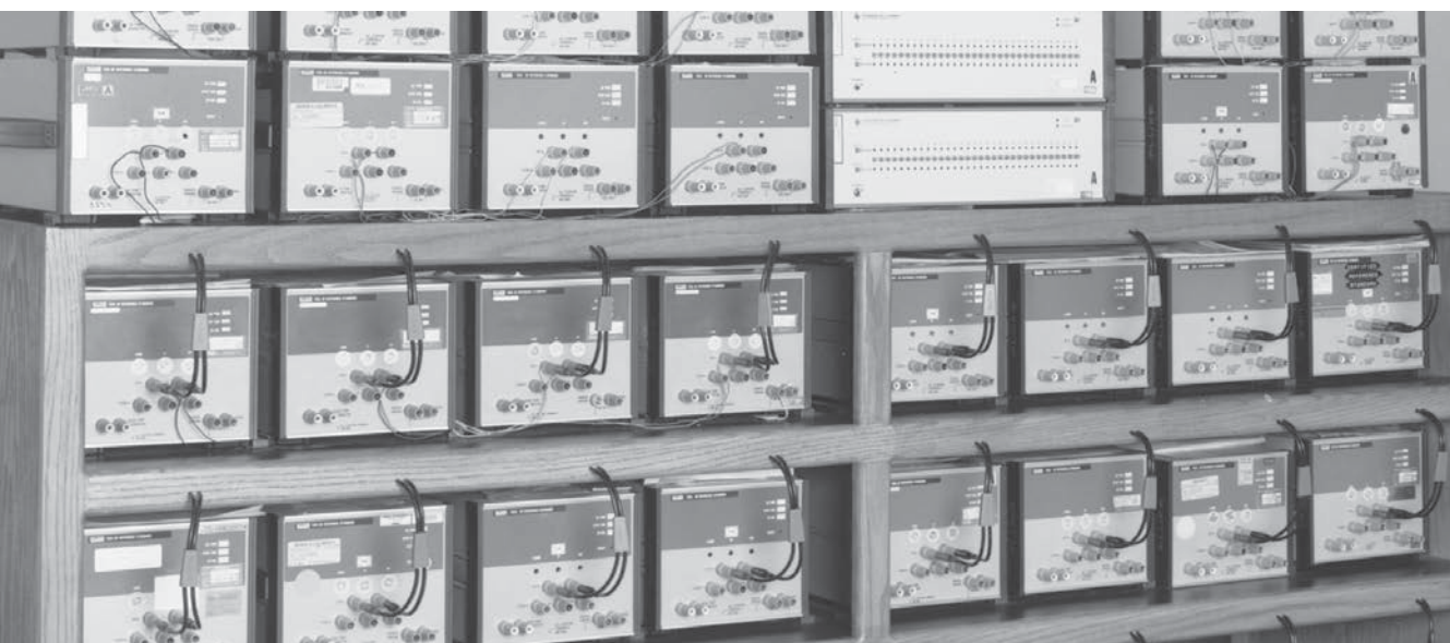
Figure 3. Several 732As and 732Bs support the Fluke Direct Voltage Maintenance Program with \pm 0.35 ppm absolute uncertainty, traceable to NIST.
