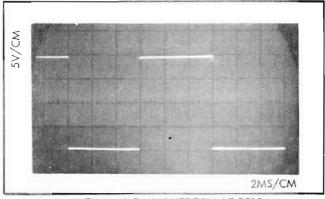
Figure 4-5. WAVEFORM AT TPIO
