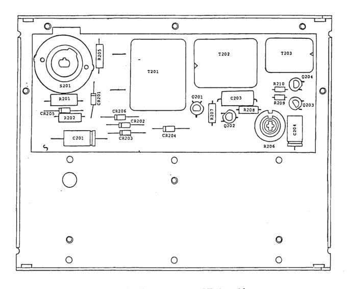
Figure 5-4. A4 Power Supply PCB Assembly
