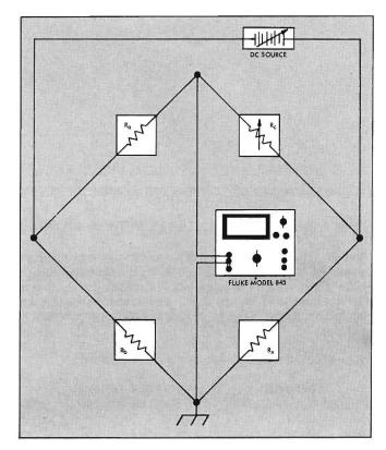
Figure 2-2. BRIDGE DETECTOR-FLOATING SUPPLY
