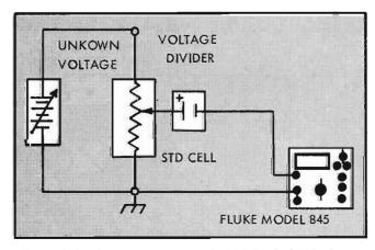
Figure 2-5. STANDARD CELL VOLTAGE MEASUREMENTS
