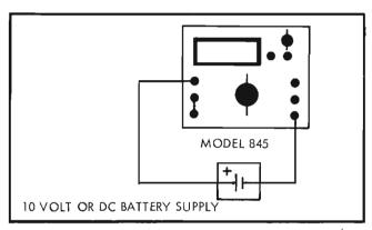
Figure 4-11. LEAKAGE RESISTANCE TEST EQUIPMENT CONNECTIONS
