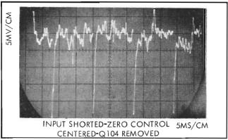
Figure 4-8. WAVEFORM AT TP2-Q104 REMOVED
