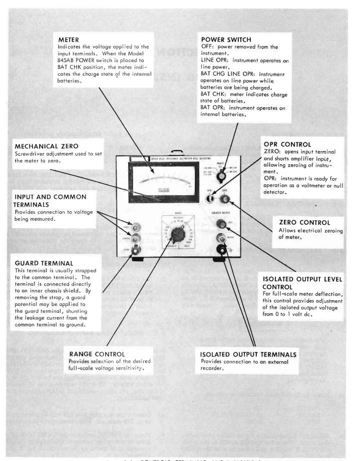
Figure 2-1. CONTROLS, TERMINALS, AND INDICATORS
