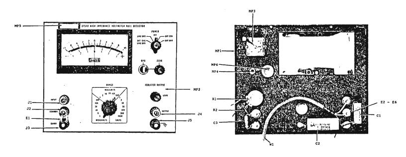
Figure 5-2. A2 Front Panel Assembly
