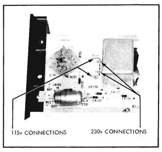
Figure 4-3. T201 115/230 VOLT AC POWER TERMINALS
