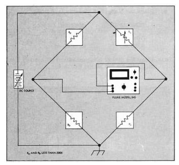
Figure 2-4. BRIDGE DETECTOR-FLOATING NULL DETECTOR
