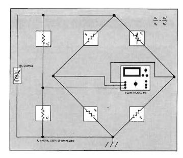
Figure 2-3. BRIDGE DETECTOR-HIGH RESISTANCE
