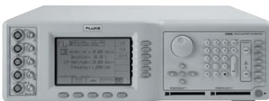
High accuracy calibration of analog and digital-storage oscilloscopes up to 3.2 and 6 GHz
