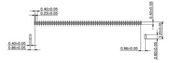
Recommended metal mask pattern Metal mask thickness: When 120µm (Terminal portion opening area ratio: 86%) (Terminal portion opening area ratio: 100%)
