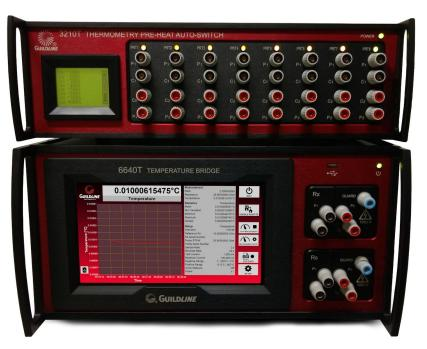
means that the 6640T is specifically **tested** at the **lower currents** (1 mA) found in thermometry and the calibration coefficients are stored separately for each decade of resistance and for each ratio. In contrast competitive DCC temperature bridges are all calibrated and specified for 10 mA to 150 mA of operation, rather than the 1 mA required for temperature measurements.
