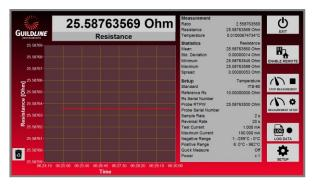
All 6640T Bridges now provide a full 10<sup>1/2</sup> digits of resolution and the ability to **graphical see** the data (trending). You can have the data presented in a **summary or detailed format** right on the Bridge Screen or available via PC based BridgeWorks Software. Measurement and **Uncertainty Analysis** you need as a Metrologist or to meet the requirements of ISO 17025 Accreditation!
