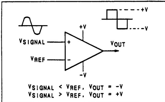
Figure 8-23. Non-Inverting Comparator
