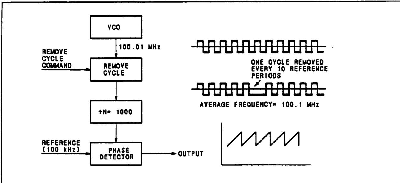
Figure 4. The Basic Block Diagram of a Modified Divide-by-N Loop With a Pulse Remover Added to Allow the VCO to Operate at a Fractional Frequency
