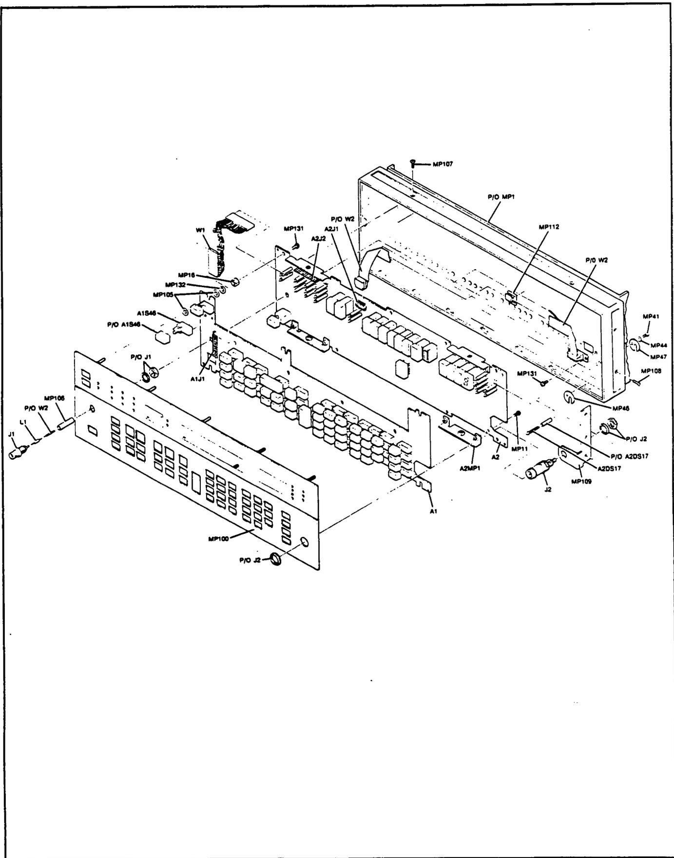
Figure 6-2 (2511A and above). Front-Panel, Parts Identification
