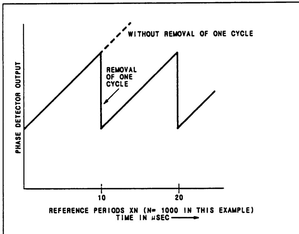
Figure 3. The Output of the Phase Detector Shown. Here is a Sawtooth Riding on a dc Voltage.
