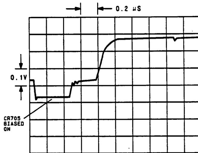
Figure 5. Oscilloscope Display between diodes CR704 and CR705 (dc coupled), Signal Generator's frequency is 950 MHz, modulation EXT FM 99 kHz (100 Hz square wave).
