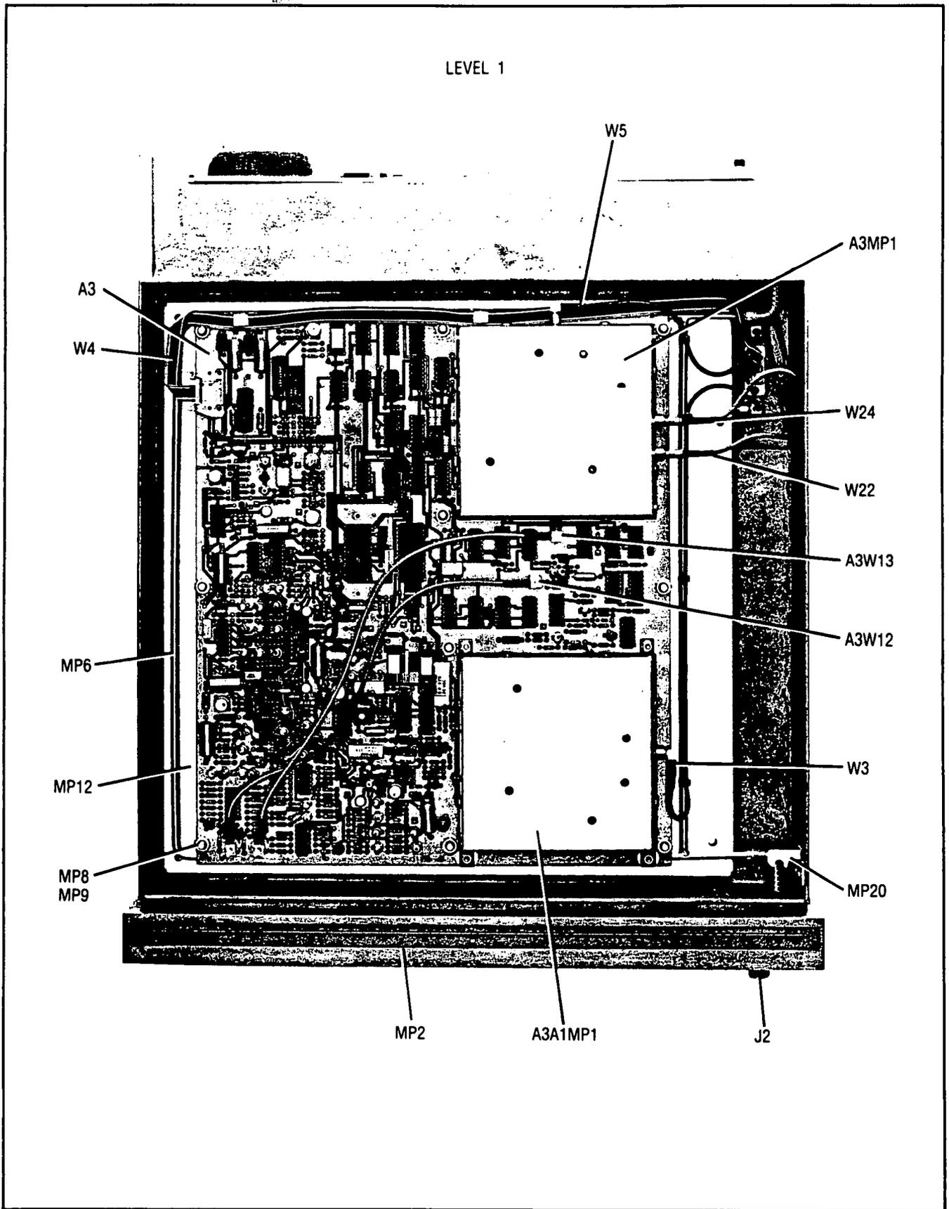
Figure 6-5 (2511A and above). Top Internal View; Top Cover Removed
