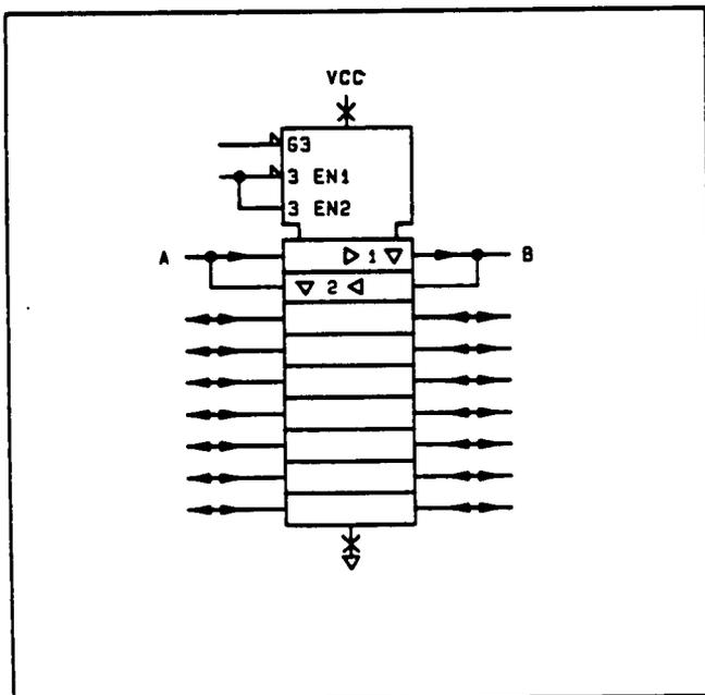
Figure 8-17. Multiple Bus Transceiver With 3-State Output
