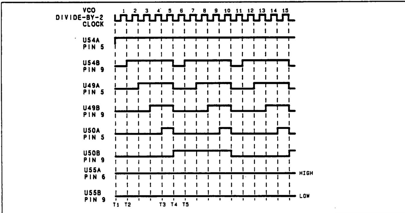
Figure 1. Divide-By-10 Timing Diagram
