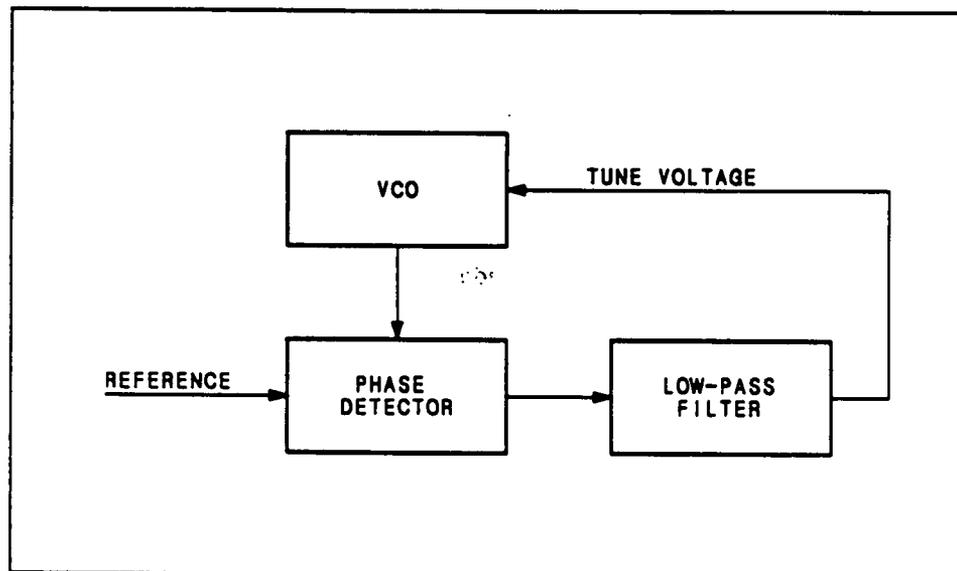
Figure 1. Basic Single Frequency Phase Lock Loop
