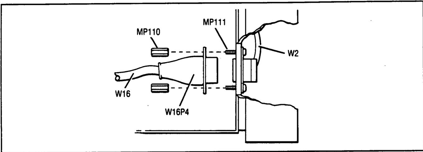
Figure 8-1.1 P/O A10/A11 Assembly Service Positioning
