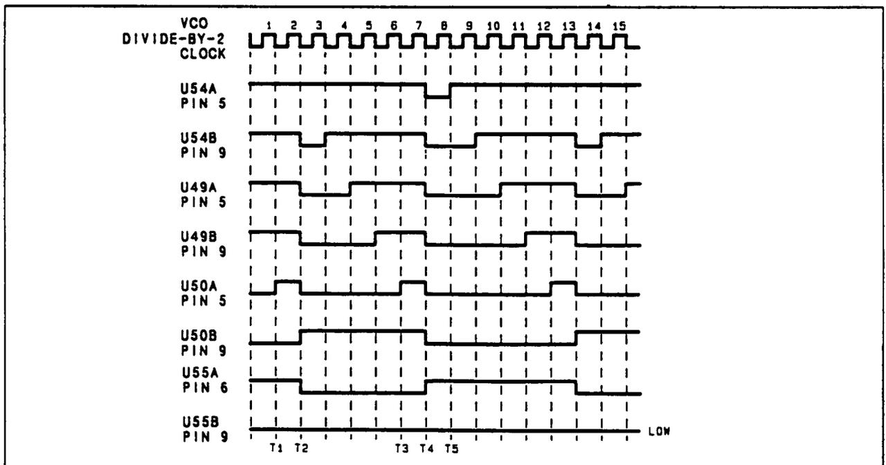
Figure 2. Divide-By-11 Timing Diagram
