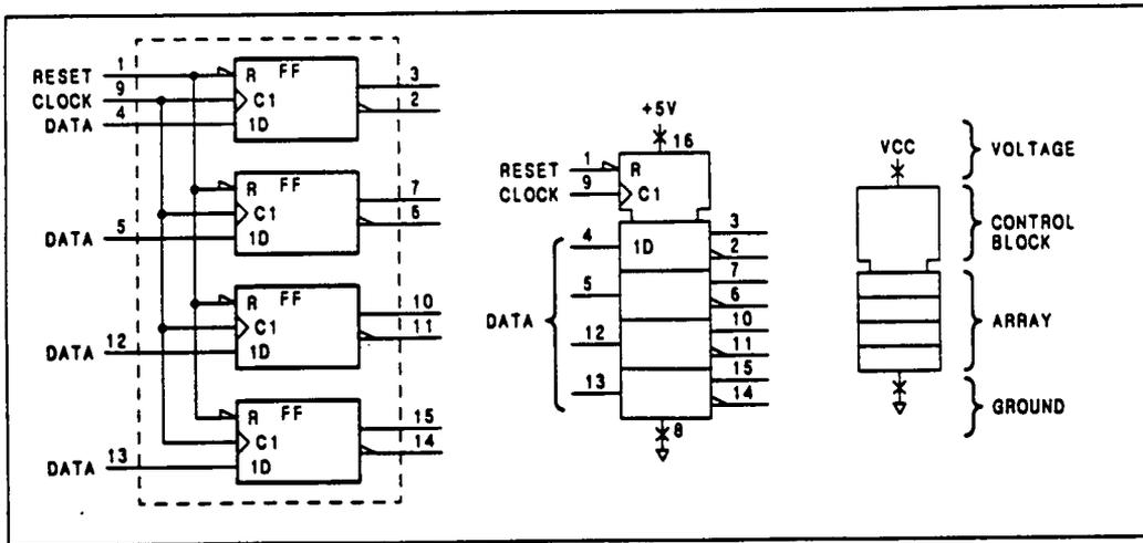
Figure 8-10. Common Control Block
