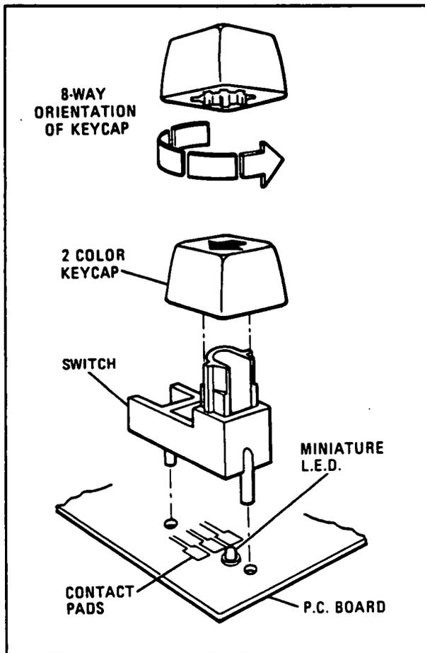
Figure 8-3. Front-Panel Pushbutton Switch Assembly
