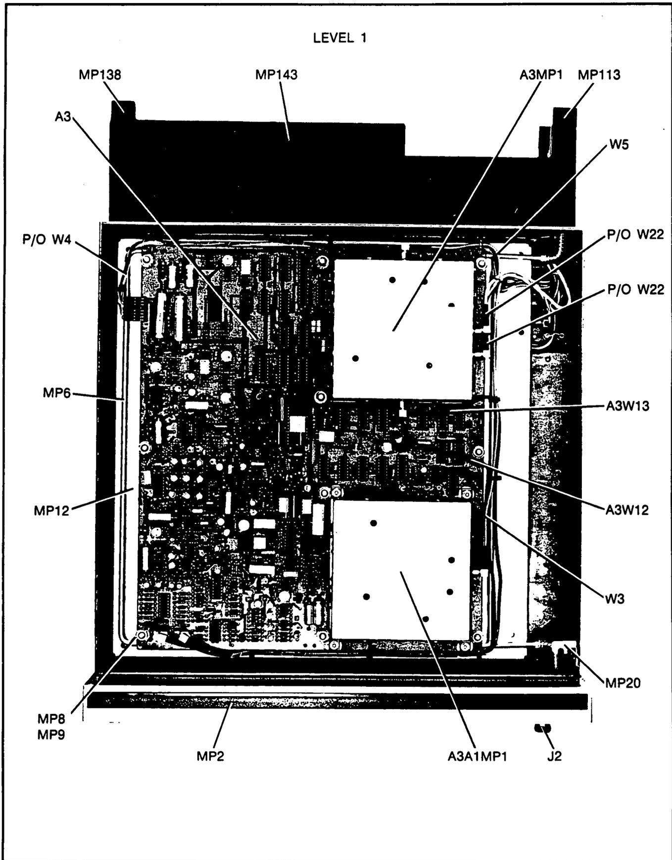
Figure 6-5 (2425A to 2509A). Top Internal View; Top Cover Removed
