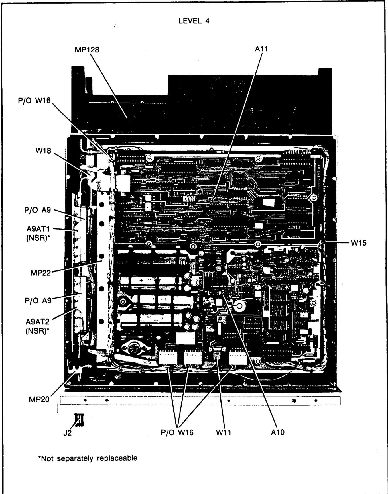
Figure 6-8 (2425A to 2509A). Bottom Internal View; Bottom Cover Removed
