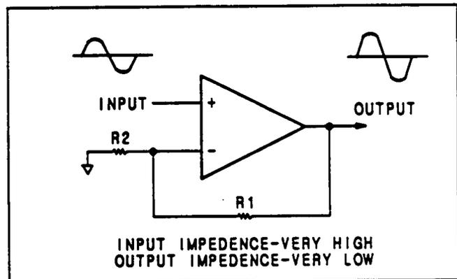
Figure 8-21. Non-Inverting Amplifier (Gain =  $1 + R1/R2$ )
