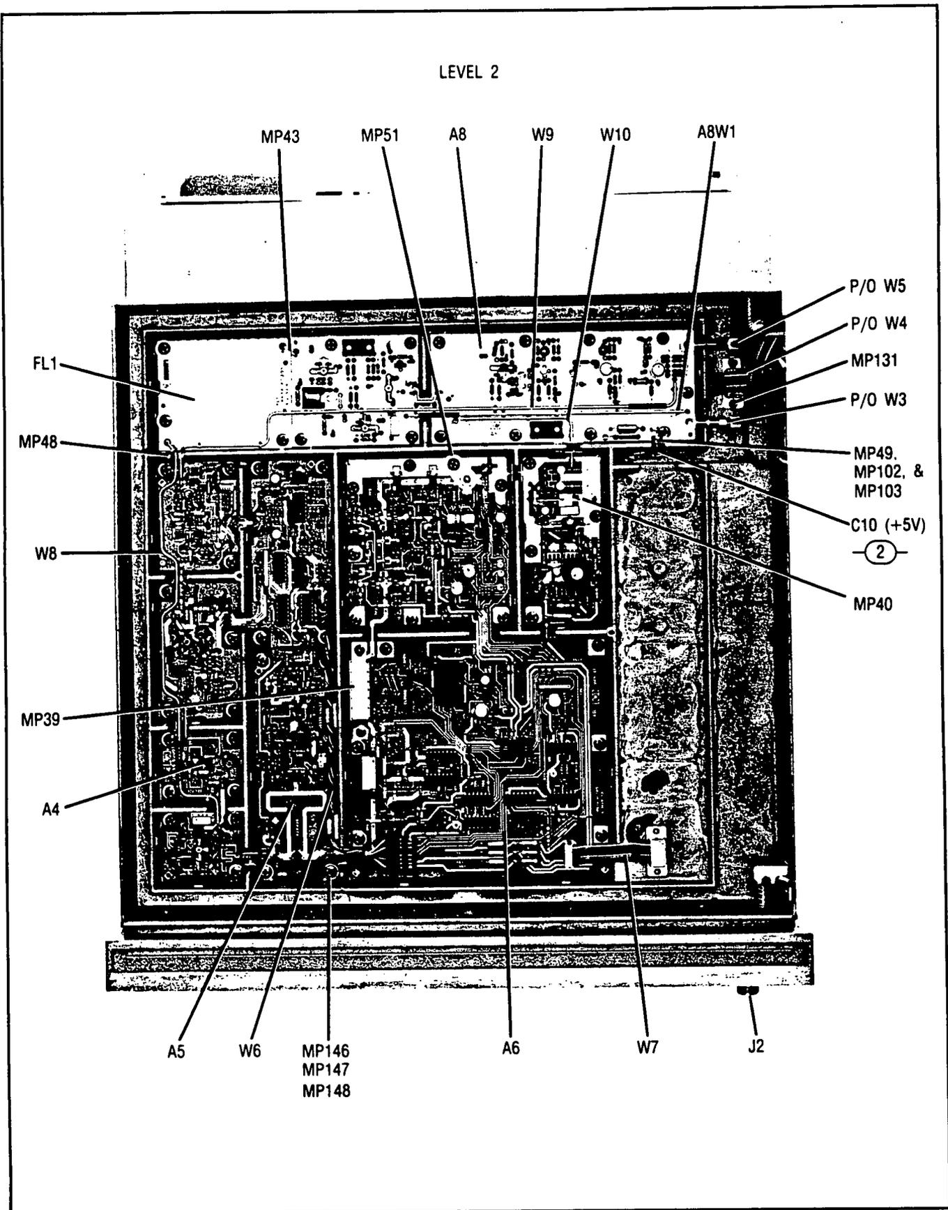
Figure 6-6 (2511A and above). Top Internal View; A3 Assembly in Service Position
