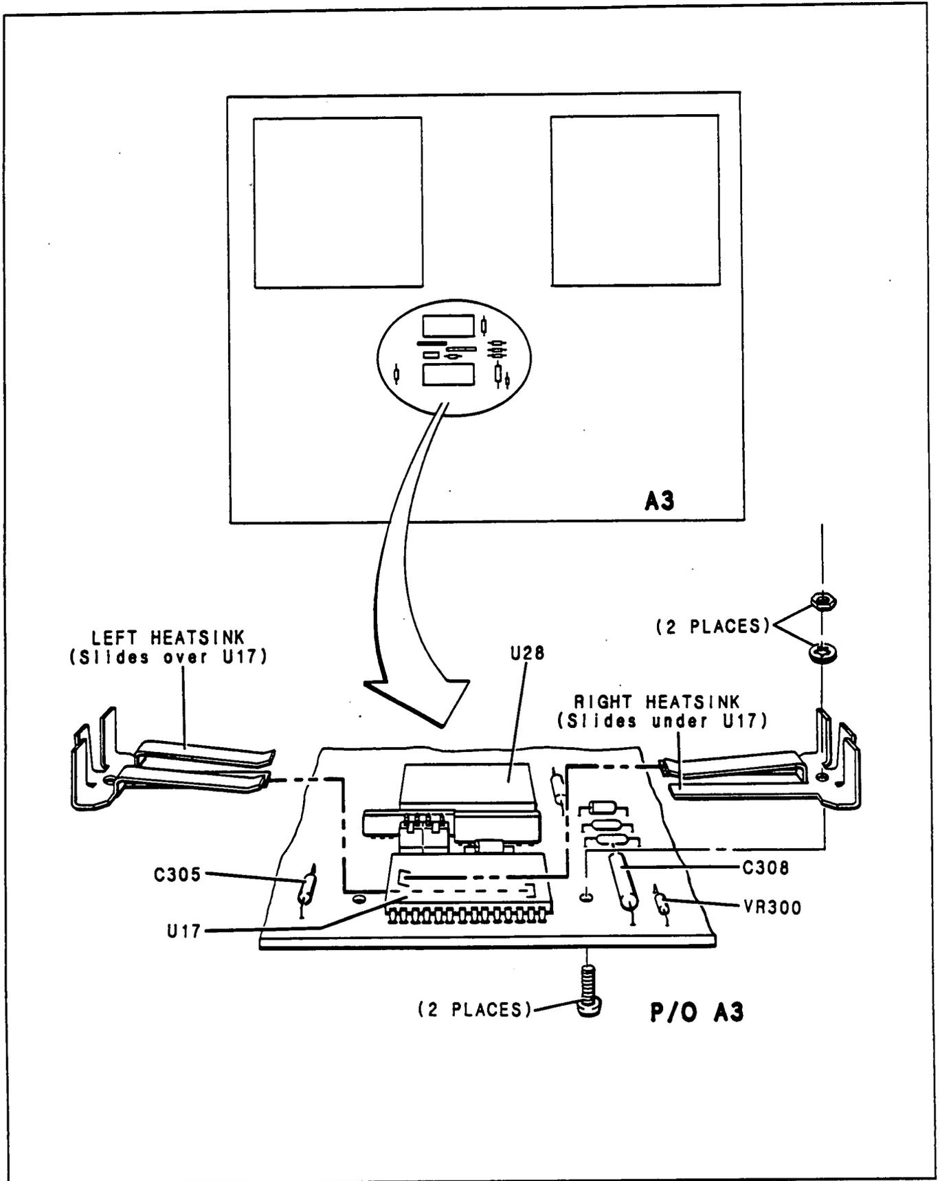
Figure 6-4 (2617A and above). Low Frequency Loop Assembly-A3, Parts Identification
