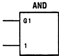
The input that controls or gates other inputs is labeled with a C or a G, followed by an identifying number. The controlled or gated input or output is labeled with the same number. In this example, 1 is controlled by G1.
