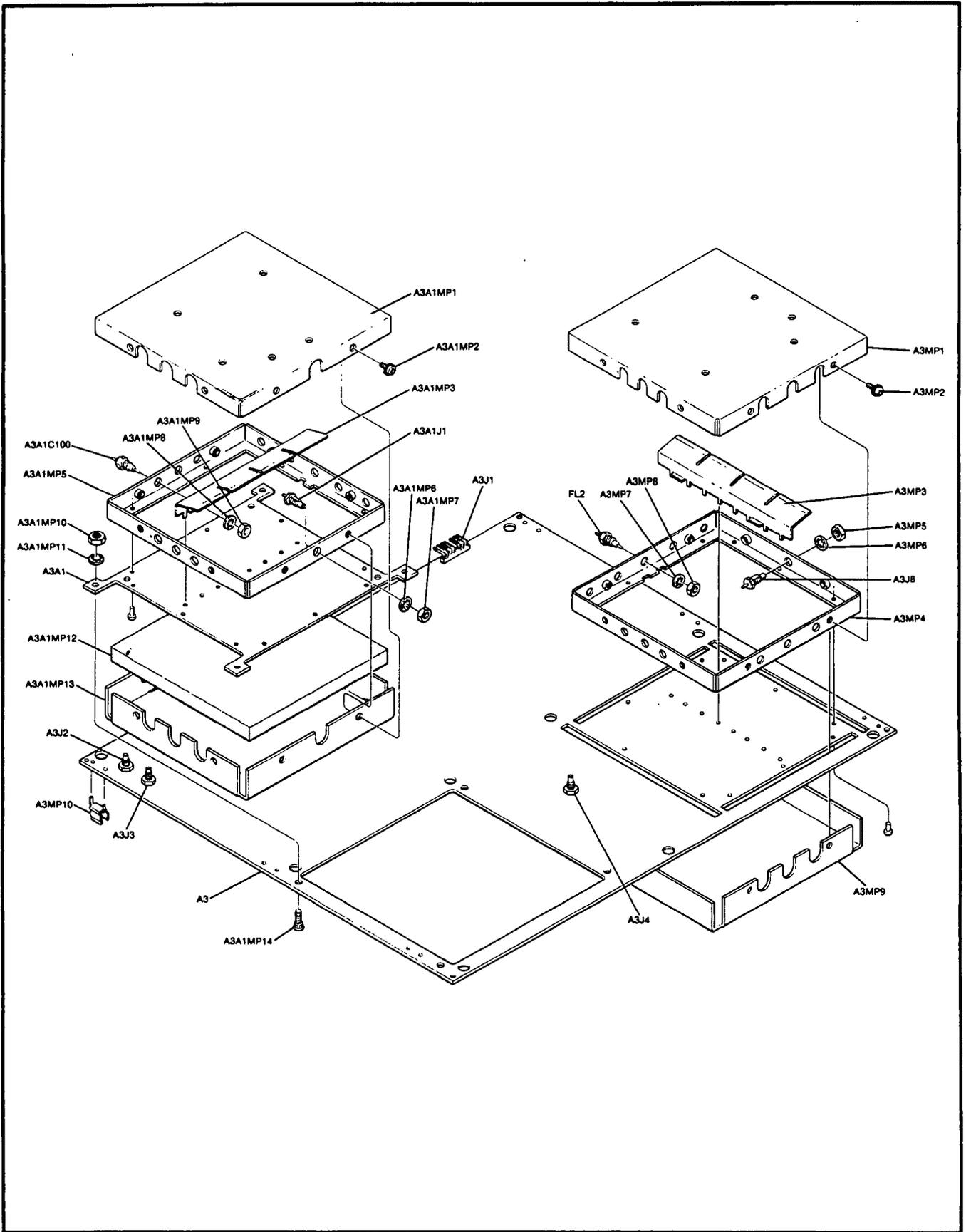
Figure 6-4 (2425A to 2509A). Low Frequency Loop Assembly—A3, Parts Identification
