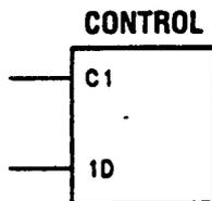
When the controlled or gated input or output already has a functional label (D is used here), that label will be prefixed by the identifying number.
