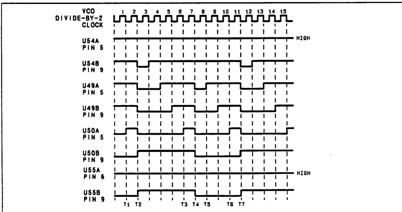
Figure 3. Divide-By-9 Timing Diagram
