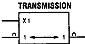
When the X1 input is active, the associated input-output pair are bi-directionally connected together. When X1 is inactive, the connection is broken.
