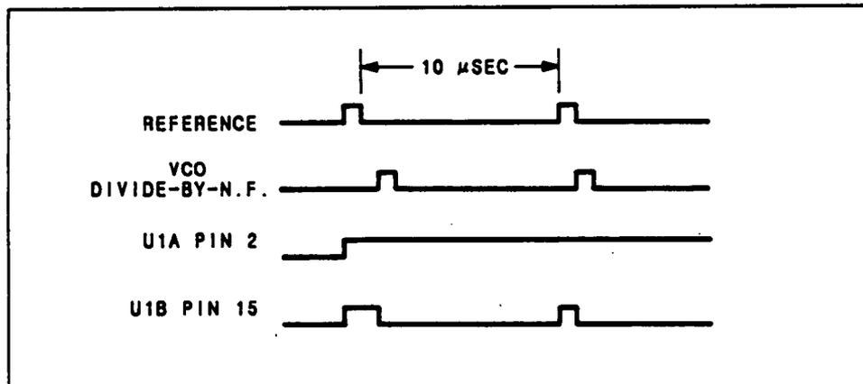
Figure 2. Timing Reference Leads VCO Divide-By-N.F.
