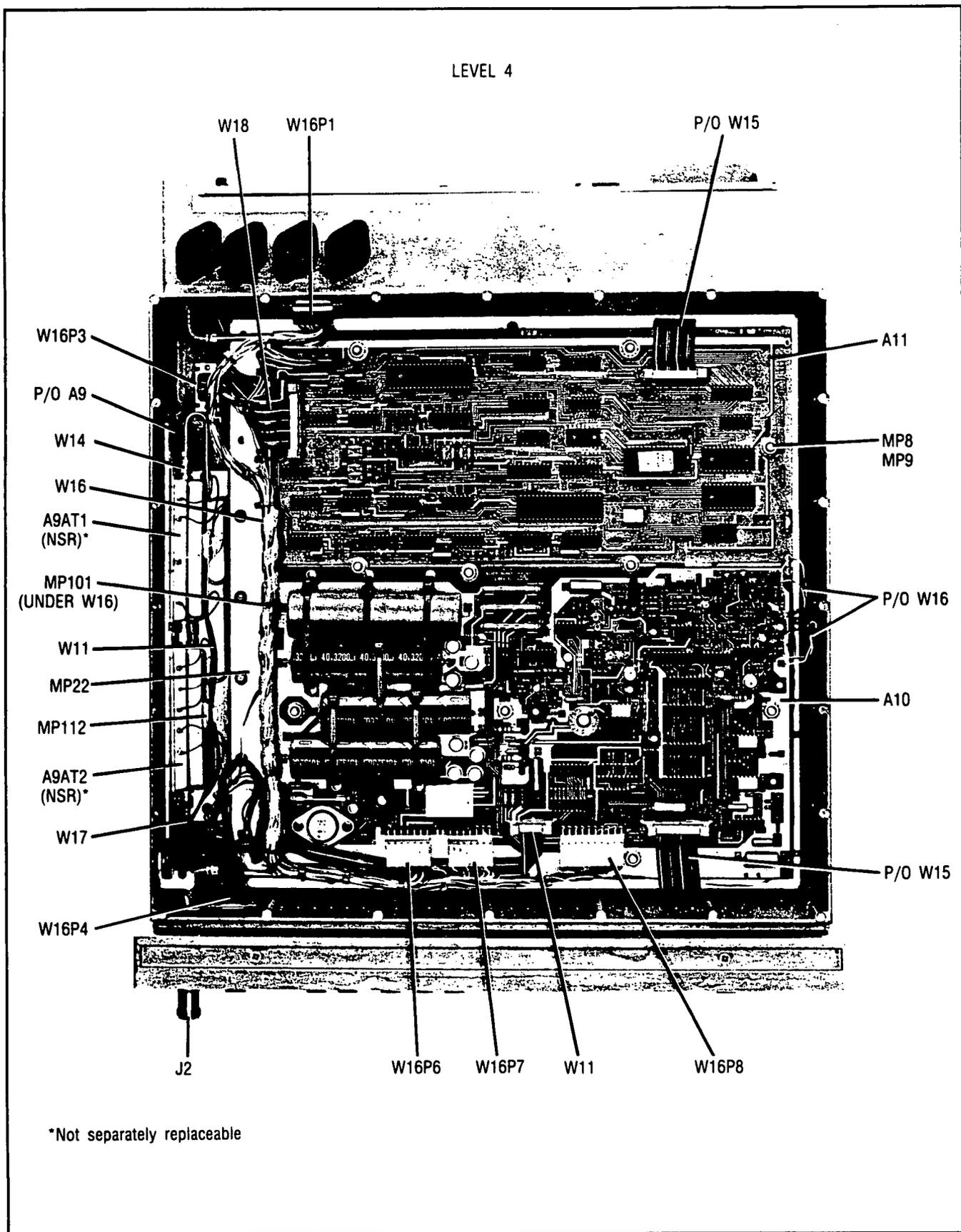
Figure 6-8 (2511A and above). Bottom Internal View; Bottom Cover Removed
