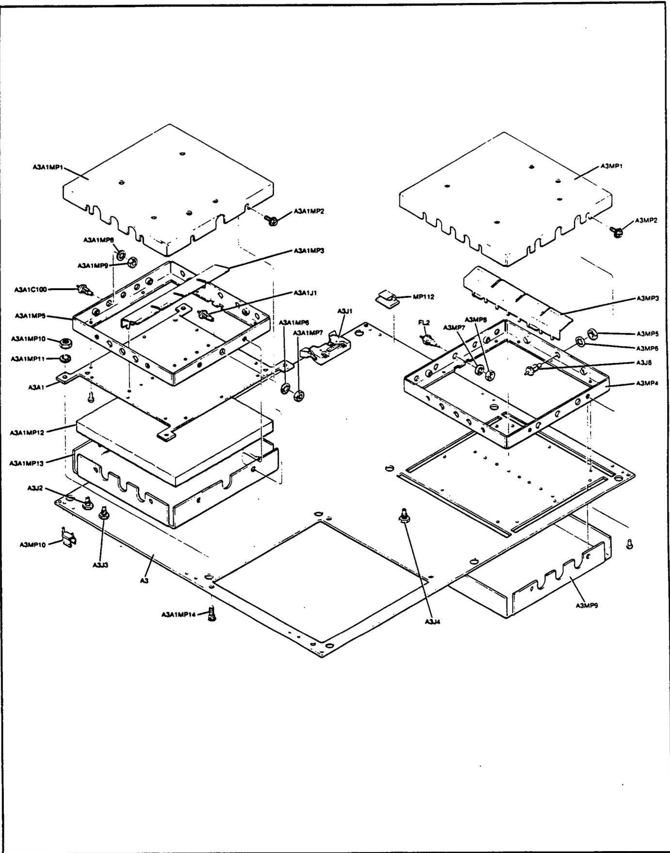
Figure 6-4 (2511A and above). Low Frequency Loop Assembly—A3, Parts Identification
