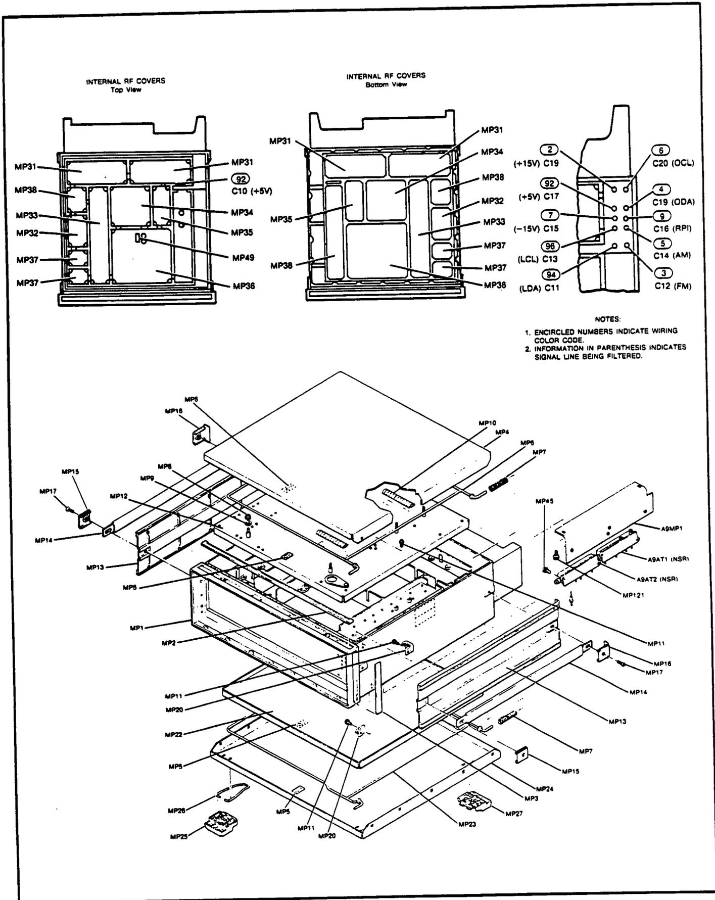
Figure 6-1 (2425A to 2509A). Cabinet, Parts Identification
