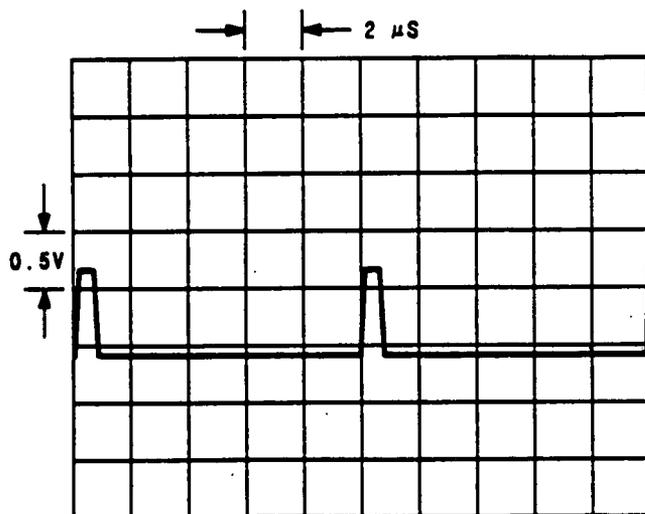
Figure 6. Oscilloscope Display of TP12 (dc coupled), W3 in W3A position, Low Frequency Loop locked, Signal Generator's frequency 990 MHz.
