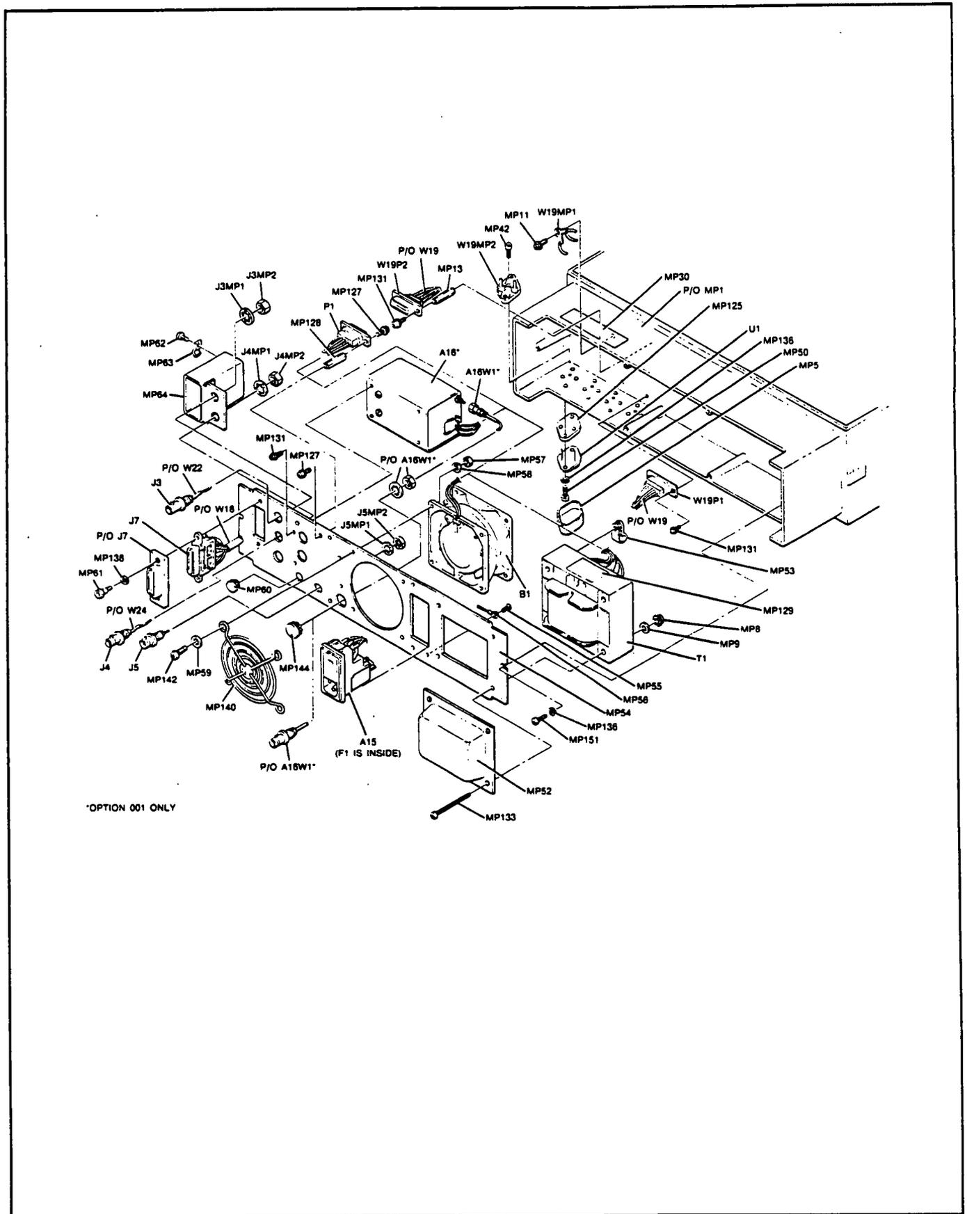
Figure 6-3 (2511A and above). Rear-Panel, Parts Identification
