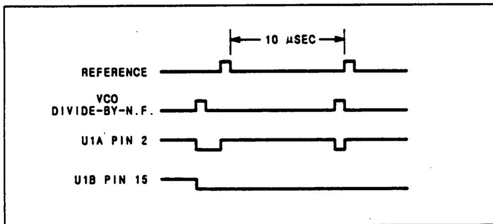
Figure 1. Timing VCO Divide-By-N.F. Leads Reference
