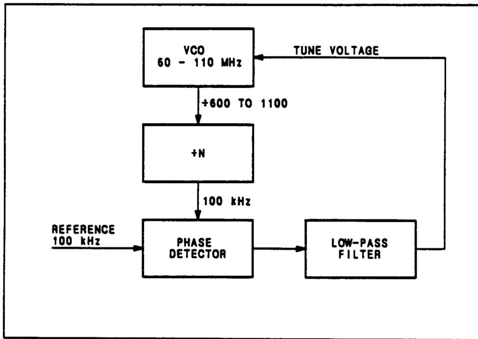
Figure 2. Basic 100 kHz Step Phase Lock Loop
