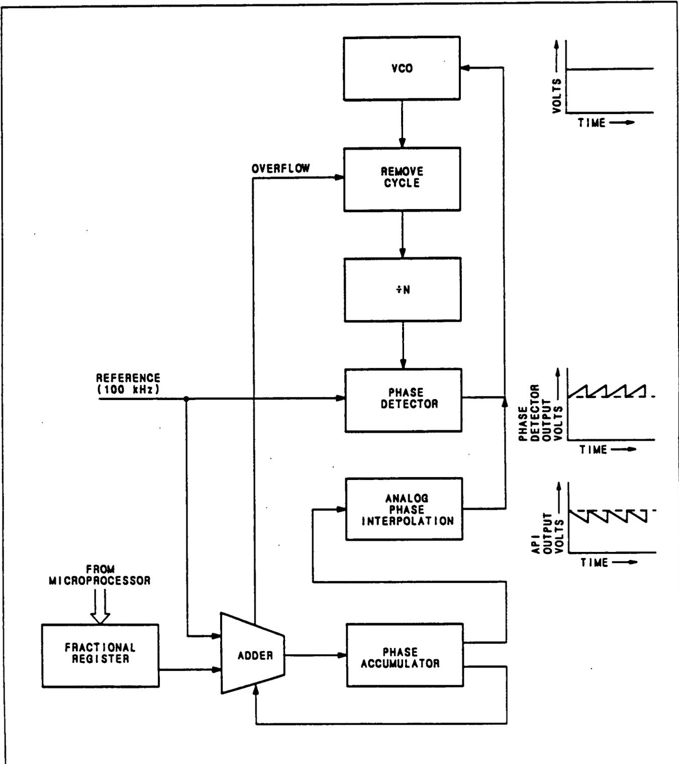
Figure 7. Simplified Diagram of a Fractional-N Phase Lock Loop
