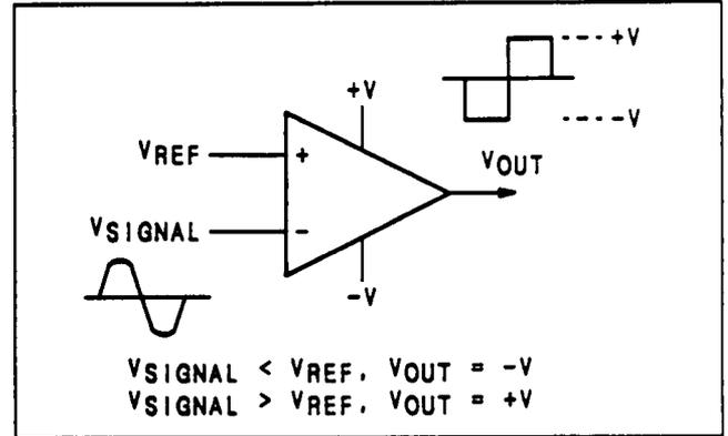
Figure 8-24. Inverting Comparator
