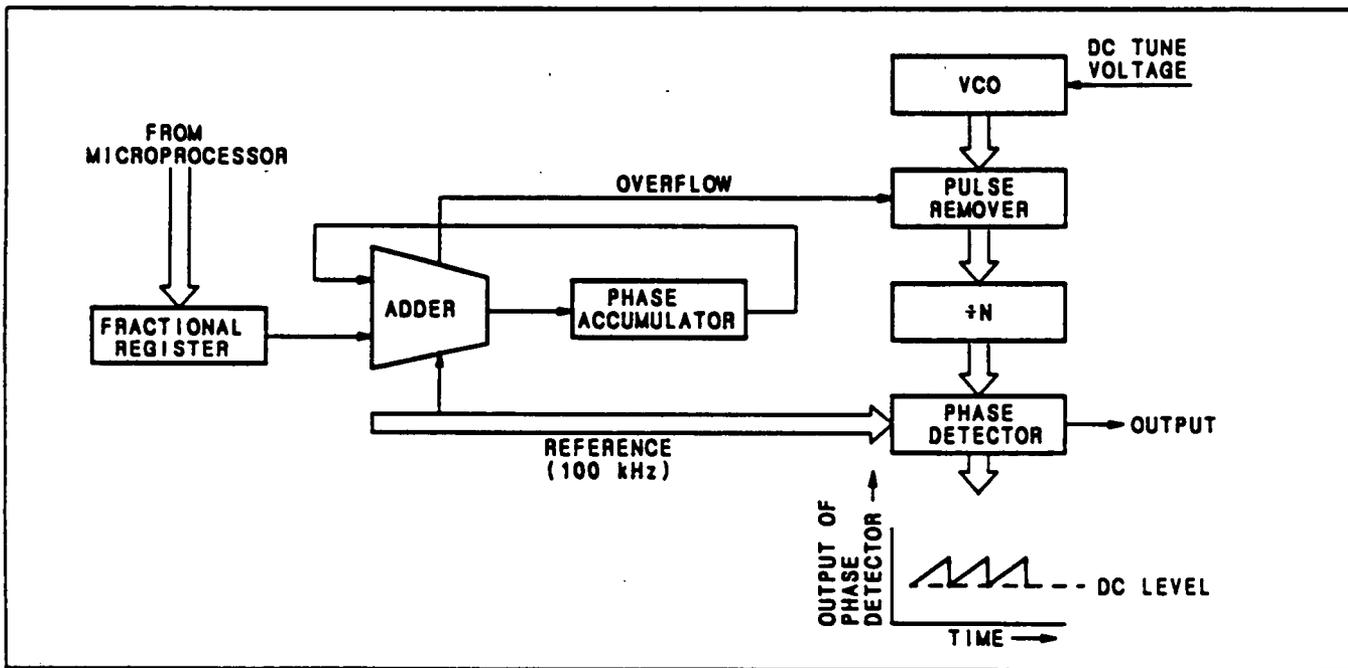
Figure 5. Fractional-N Loop Showing a Phase Register Used to Trigger the Removal of one VCO Cycle (or Pulse)
