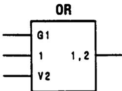
When a V input is active, the output will be in its active state. With the V input inactive, the device functions as if the V input doesn't exist.
