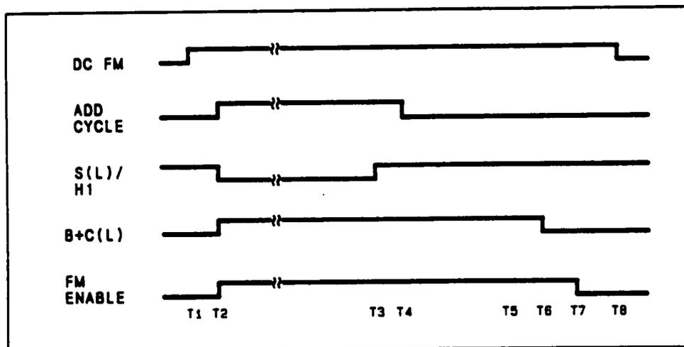
Figure 1. FM Calibration Timing Diagram
