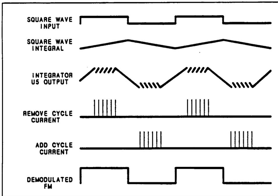
Figure 1. 10 Hz Square Wave In-Band Modulation
