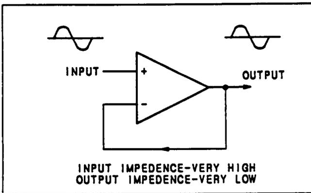
Figure 8-20. Non-Inverting Amplifier (Gain = 1)
