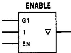
When the EN input is active, the output is enabled to function normally. When the EN input is inactive, the three-state output (  $\nabla$  ), in this case, becomes a high impedance, effectively removing that device from the circuit.
