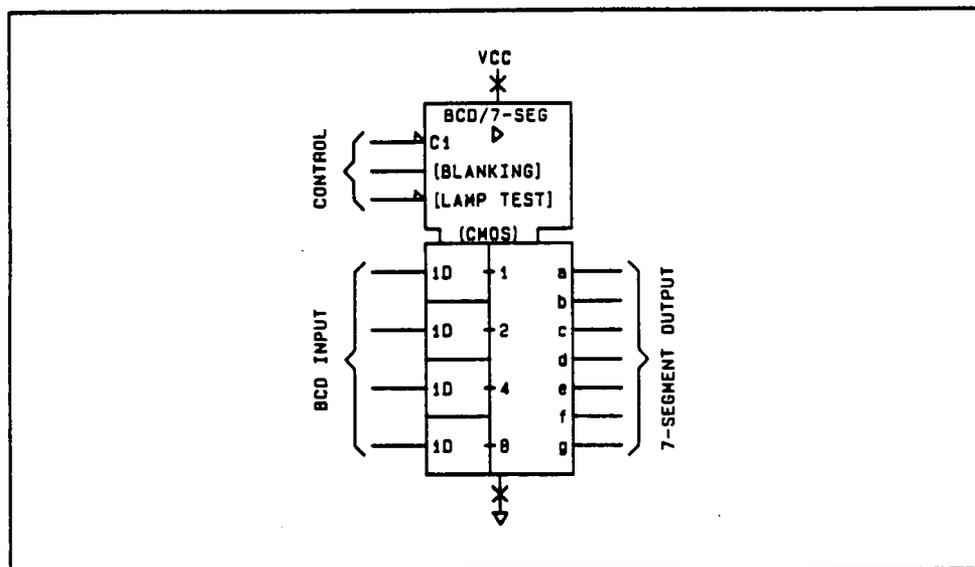
Figure 8-19. BDC-to-Seven-Segment Latch/Decoder/Driver
