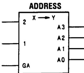
When GA is active, the active address line (0 through 3) is the decoded value of the 1 and 2 binary inputs. When the controlled address lines have a functional value, that value will be prefixed by the identifying letter.
