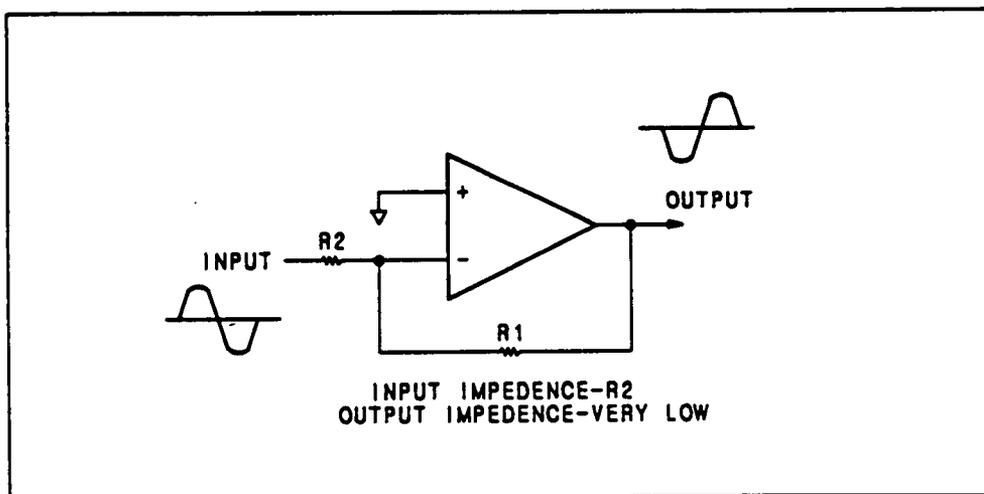
Figure 8-22. Inverting Amplifier (Gain =  $-R1/R2$ )
