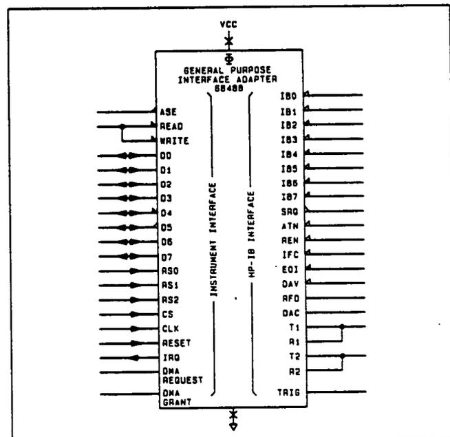
Figure 8-18. General Purpose Interface Adapter
