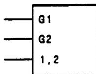
If the input or output is affected by more than one gate or control input, then the identifying numbers of each gate or control input will appear separated by commas.
