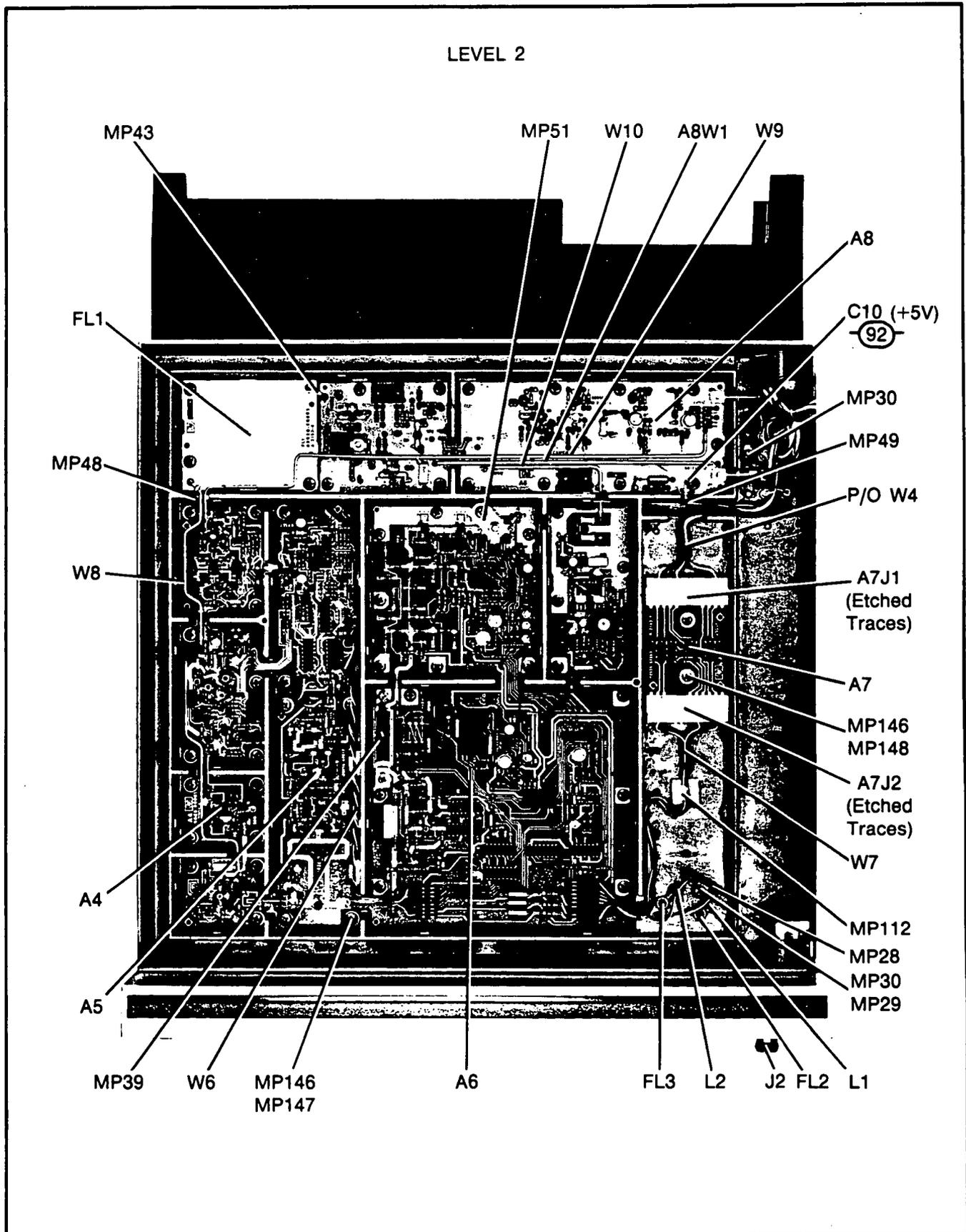
Figure 6-6 (2425A to 2509A). Top Internal View; A3 Assembly in Service Position
