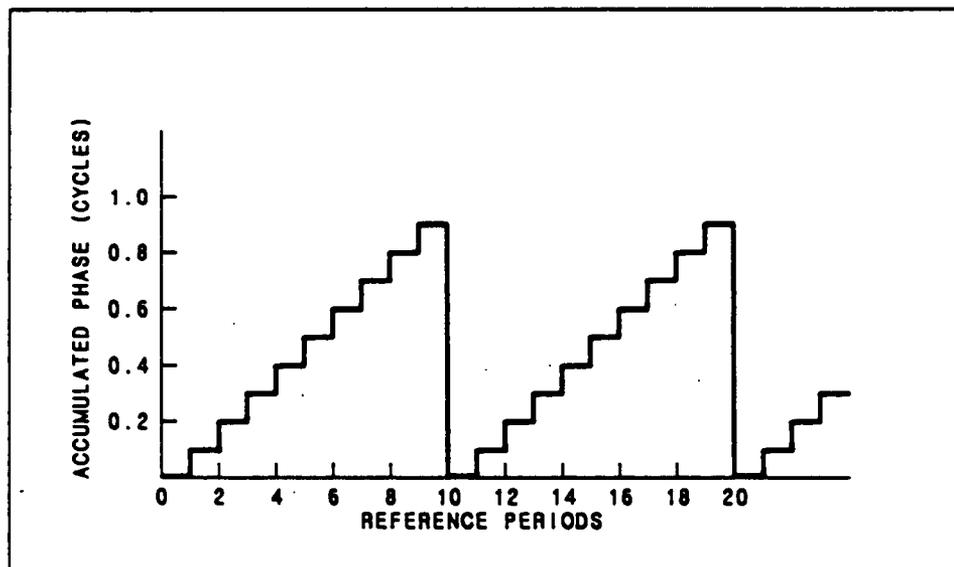
*Figure 6. Phase Detector Waveform*
