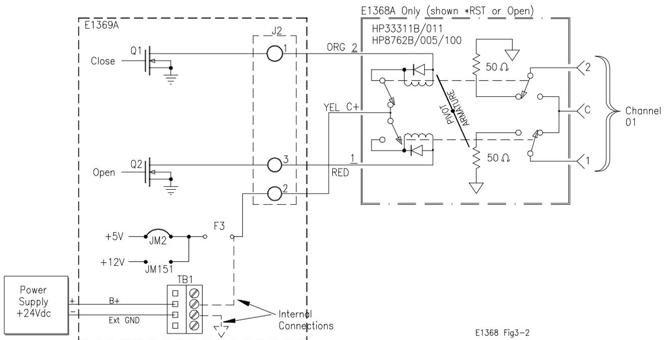
Figure 3-2. Example: Single Channel Switching using External Power
