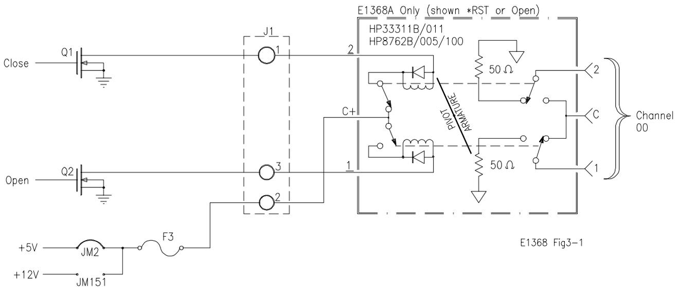
Figure 3-1. Example: HP E1368A Single Channel Switching
