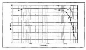
Fig. 2. Typical response of -bp- 460A Amplifier working into (B) resistive load (A) using -bp- 410A Voltmeter (C) Gaussian curve.
