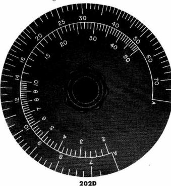
The -hp- Model 202D is a modification of the 200D, which extends the range down to 2 cps. The tuning dial is calibrated over approximately 300°; the effective scale length is about 75". Before calibration, all -hp- Audio Oscillators are operated for a long period so as to be completely stabilized.
