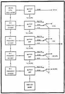
Fig. 1. Block diagram of circuit, Model 100D.
