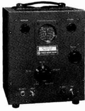
This new -hp- instrument is a super-regenerative (AM) receiver covering all frequencies between 10 and 500 mc in 5 bands. It is designed for use with the -hp- 803A Bridge. It offers a high sensitivity of 5 microvolts over the entire frequency band. It is designed for fast, simple operation, and has a single, convenient frequency control directly calibrated in megacycles.
