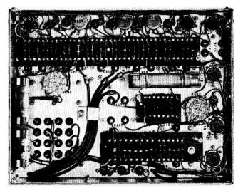
Fig. 1 — Rear view of -hp- 616A UHF Signal Generator, showing compact arrangement and ready accessibility of all components.
