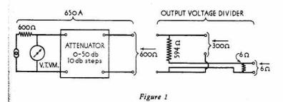
Circuits of the -hp- Model 650A have been carefully proportioned and low temperature coefficient components have been employed to assure highest frequency stability. Output voltage will remain constant over long periods of time, despite wide variations in temperature. Distortion over the low frequency bands is kept at a minimum to increase the usefulness of the instrument for audio measurements.
