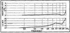
Fig. 2. Typical band pass characteristics.
