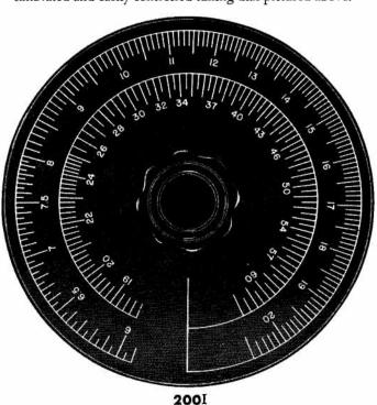
Main tuning dial of the 200I, which is an oscillator of the band-spread type, intended for comparison work. The dial is calibrated over approximately 300° with effective scale length about 90" and range of 6 cps to 6 kc. Each Model 200I is carefully hand calibrated to insure maximum accuracy.
