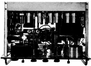
Fig. 2 —Top view of signal generator showing klystron oscillator cavity and bolometer circuits. Aperture at right permits easy replacement of oscillator tube.
