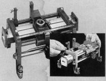
Convenient, all-purpose -hp- 809B carriage operates with six different -hp- slotted sections, waveguide and coaxial. Mounts sections covering frequencies 3,000 to 18,000 mc—sections interchange in 30 seconds! Precision-built carriage calibrated in mm to 0.1 mm; dial gauge may be mounted. Operates with -hp- 442B Broad Band Probe and -hp- 440A Coaxial Detector in combination; or with -hp- 444A Untuned Probe.
