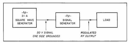
Figure 4: Typical set-up for applying modulation to -hp- signal generators.
