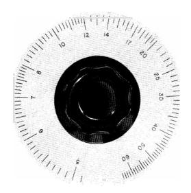
Main tuning dial of -hp- Model 200CD is calibrated over approximately 300° and has an effective scale length of about 60° inches. This precisely calibrated dial with its easy-to-use control contributes much to the accuracy and convenience of the wide-range Model 200CD oscillator.
