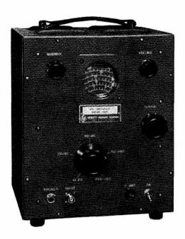
This -hp- instrument is a super-regenerative (AM) receiver covering all frequencies between 10 and 500 MC in 5 bands. It is designed for use with the -hp- 803A Bridge. It offers a high sensitivity of 5 microvolts over the entire frequency band. It is designed for fast, simple operation, and has a single, convenient frequency control directly calibrated in megacycles.
