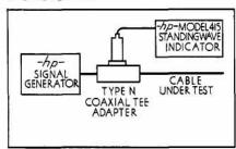
Figure 3. Arrangement of instruments for measuring velocity of propagation.
