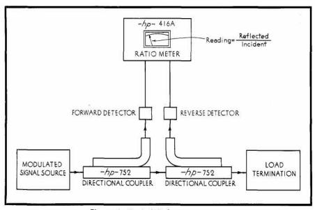
Figure 4: Typical Reflectometer set-up.
