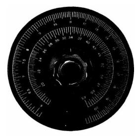
Main funing dial of -hp- Model 200I, a band-spread oscillator designed for comparison work. The dial is calibrated over approximately 300° with effective scale length of about 90 inches and range of 6 cps to 6 KC. Each instrument is carefully hand-calibrated for maximum accuracy.
