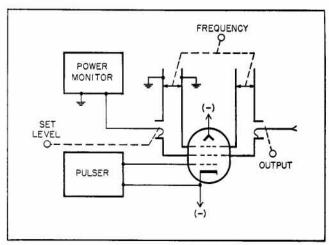
Figure 1. Block Diagram, -hp- 614A Signal Generator.
