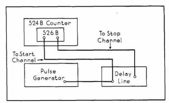
Figure 2. Measurement of time delay of a delay line with -hp-524B Electronic Counter and -hp-526B Time Interval Unit.
