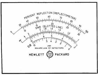
Figure 2. Meter scale, -hp- 416A Ratio Meter. Note that meter has separate scales for percentage reflection, SWR, and db.
