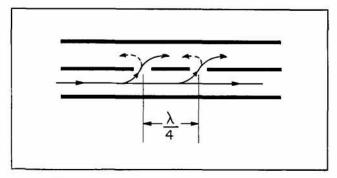
Figure 2. Cross-section, two-aperture coupler.
