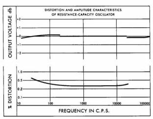
Figure 2. Distortion and Amplitude Characteristics, RC Oscillator.
