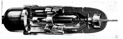
Figure 1. Construction details of -hp- diode probe.
