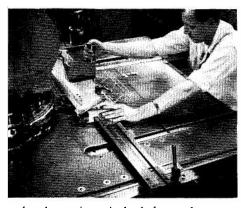
Another unit typical of the modern machinery in daily use at -hp- is this turret press, a precision equipment which punches many sizes of perforations on instrument chassis with a single setup.
