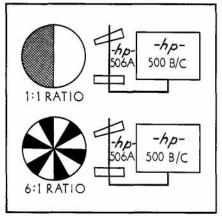
Figure 3. Typical setup for extending low-frequency range of -hp- 500B/C Electronic Tachometer Indicators.
