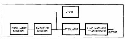
Figure 1. Elements of a signal generator.
