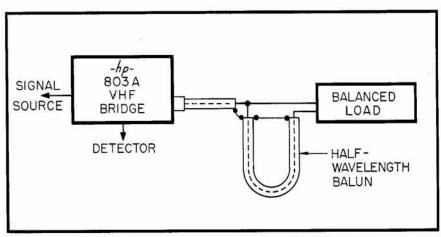
Figure 6: Measurement set-up using balun with balanced load.
