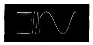
Figure 1. Oscillogram shows freedom from transients as output frequency is rapidly changed.
