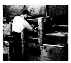
The -hp- plant is equipped with the most modern manufacturing machinery available for the job. Here is a heavy duty die casting machine for production of housings, shields, dials and other cast parts.
