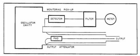
Figure 5: Monitoring and Attenuating system in -hp- signal generators.
