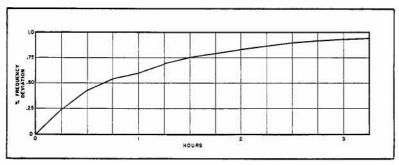
Figure 6. Short-time Stability Curve of RC Oscillator.
