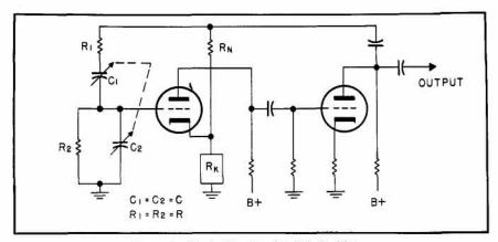
Figure 1. Basic Circuit, -hp- RC Oscillator.
