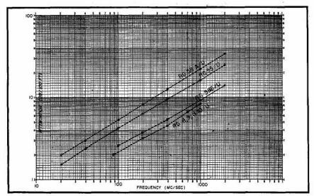
Figure 9: Attenuation vs. frequency curves for several cables.
