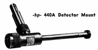
A simple, easily used instrument for detecting rf energy in coaxial or waveguide systems. In coaxial use, covers all frequencies 2.4 to 12.4 KMC. Uses either 1N21 or 1N23
