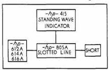
Figure 2. Suggested instrument arrangement for measuring small values of cable attenuation. Unknown cable is placed between slotted line and short.
