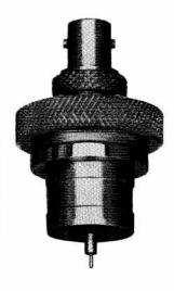
A 1N26 crystal plus a small antenna in a convenient housing permitting probe penetration to be varied quickly and easily. Probe position is fixed by a locking ring. Requires no tuning; and sensitivity surpasses most elaborate single and double-tuned probes (particularly between 8.0 and 18.0 KMC). Polyiron inserts damp spurious resonances. Frequency coverage 2.4 to 18.0 KMC; modified 1N76 crystal; BNC output jack. For 3/4" mounting hole as on -hp- 809B Carriage (Page 104).
