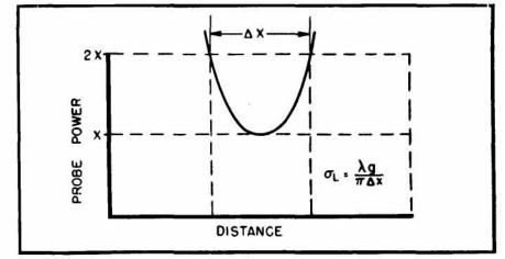
Figure 3: Twice minimum power method for measuring SWR.
