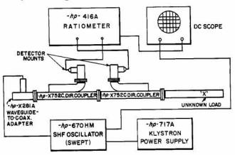
Figure 1. Typical Reflectometer Setup. Note use of two directional couplers back-to-back, with individual detectors, for simultaneous evaluation of incident and reflected powers.
