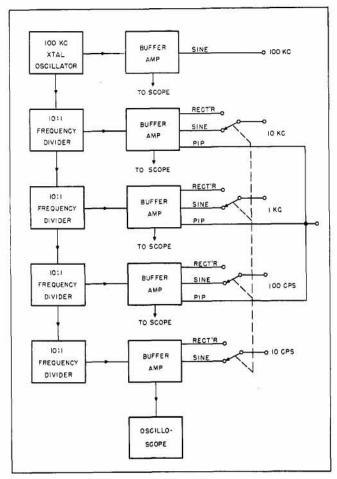
Figure 1. Block diagram of circuit, Model 100D.
