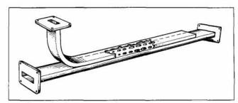
Figure 1. Construction, -hp- 752 Directional Couplers.
