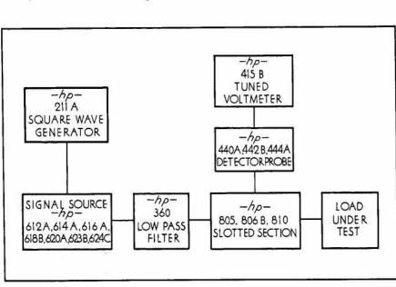
Figure 1: Typical set-up for impedance measurements.
