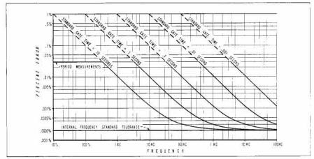
Figure 3. Possible error factor in frequency measurement (-hp- 524B, 525A).
