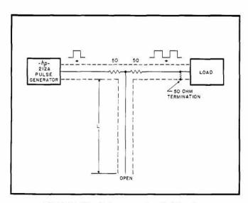
Figure 3. Circuit for generating double pulses.
