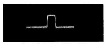
Figure 2. Typical rf pulse, 0.25 µsec, 62+C.
