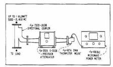
Fig. 6. Arrangement for measuring average power from 1 watt to 1 kilowatt in waveguide system.
