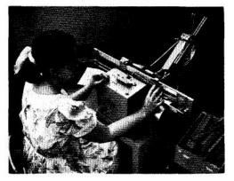
The Kingman Machine, above, is another device born and built at -hp- to make possible faster manufacturing at lower cost. Named for the -hp- engineer who "imagineered" it, it mass-produces terminal boards.
