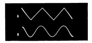
Figure 2. Oscillogram of (A) triangular wave applied to special -hp- developed shaping circuit and (B) resulting true sine wave.
