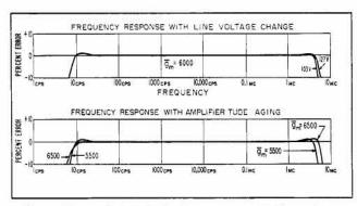
Figure 1. Typical variation in accuracy with line voltage changes and mutual conductance changes (geometric mean value of amplifier tubes).
