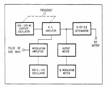
Figure 1. Block diagram, -hp- 612A uhf-TV Signal Generator.
