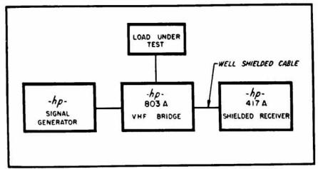
Figure 5: Impedance measurements for frequencies below 500 MC.
