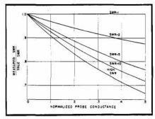
Figure 2: Effect of probe penetration on measured SWR.
