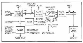
Figure 1. Simplified circuit diagram -hp- 624C Test Set.
