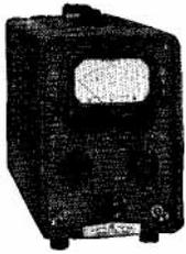
No computations! Provides instantaneous, automatic power readings *direct* in dbm or mw at all frequencies for which there are suitable bolometer mounts. For CW measurements, uses either 1/100 amp. fuse or Sperry 821 barretter. Also measures CW or pulsed power with negative coefficient thermistor. Provides up to 16 ma bias current. Operates with all mounts in adjacent table. \$250.00.
