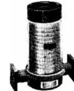
Inexpensive, general-purpose, direct-reading. Consists of high Q resonant cavity tuned by choke plunger; no sliding contacts. Full range coverage 8.2 to 12.4 KMC, accuracy 0.08%, resettability 0.01%. 1.5 db output dip indicates resonance. No backlash. \$125.00.
