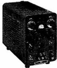
**-hp- 715A** is a versatile source of regulated beam and reflector voltage for operating most test bench klystron tubes. Beam voltage 250 to 400 v; reflector voltage 0 to 900 v; 6.3 v filament. Internal, 1,000 cps square wave modulation, also 60 cps FM modulation, both on reflector voltage. \$300.00.
