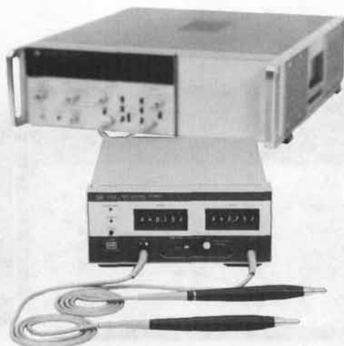
HP-IB programmable Time Interval Probes
