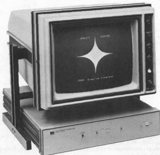
The 1350S Display System includes a 1311 X-Y Display, a 1350A Graphics Translator, an interconnecting cable, and a binder for instruction manuals.
