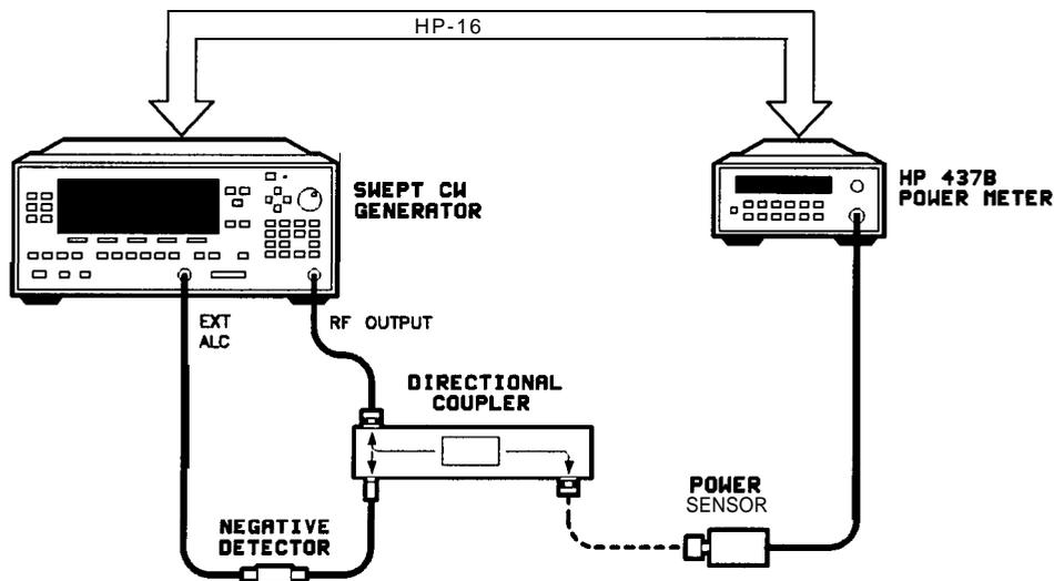
Figure 1-22. Automatically Characterizing and Compensating for a Detector
