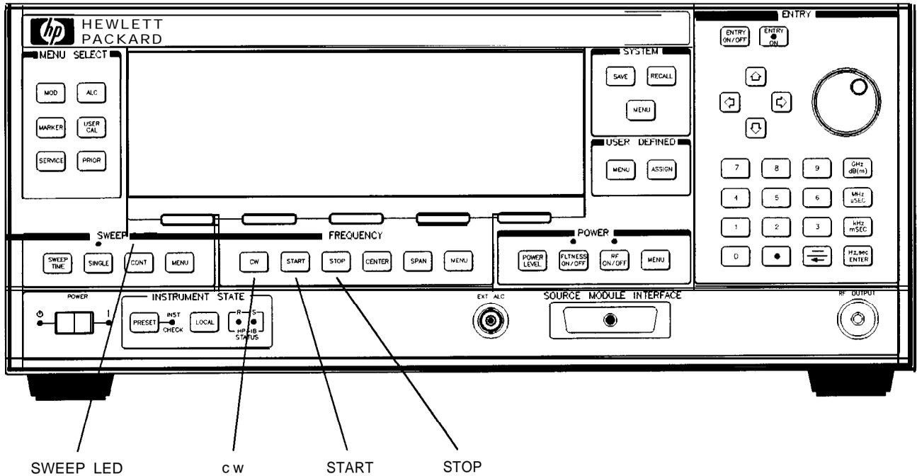
Figure 1-4. CW Operation and Start/Stop Frequency Sweep
