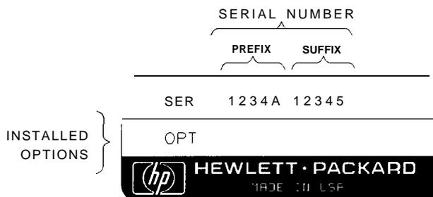
Figure O-1. Typical Serial Number Label
