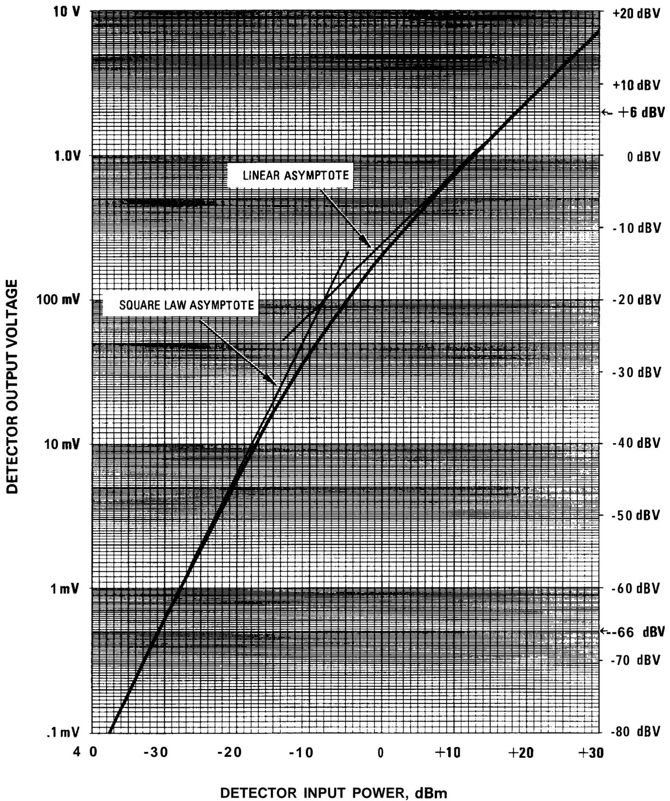
Figure 1-12. Typical Diode Detector Response at 25°C
