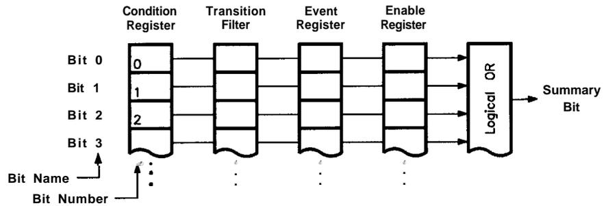
Figure I-33. Generalized Status Register Model
