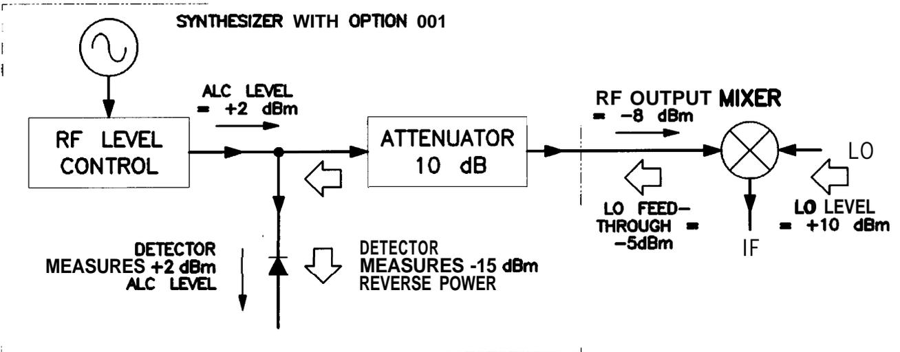
Figure 1-17. Reverse Power Effects, Uncoupled Operation with -8dBm Output
