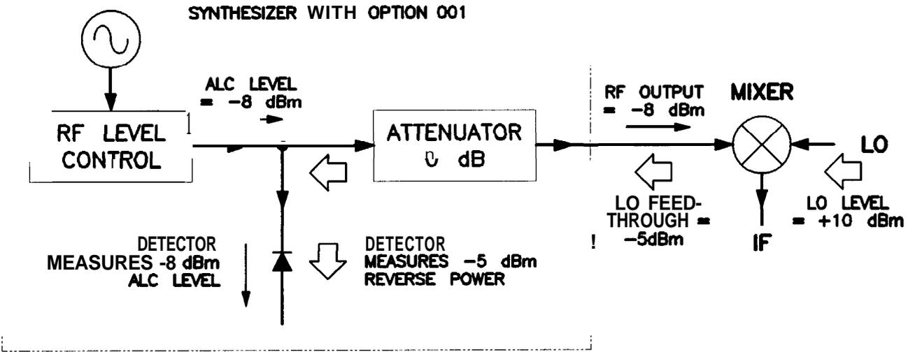
Figure 1-16. Reverse Power Effects, Coupled Operation with -8dBm Output
