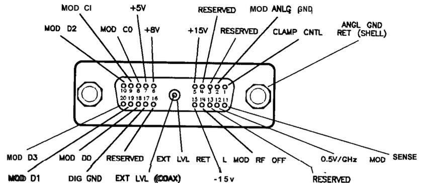
**Figure C-3. Interface Signals of the Source Module Connector**
