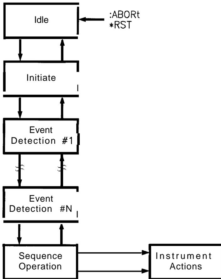
Figure I-35. Generalized Trigger Model
