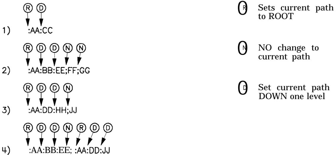
**Figure I-26. Proper Use of the Colon and Semicolon**
