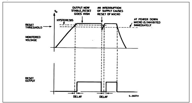
Figure 1 : Reset Output Waveforms
