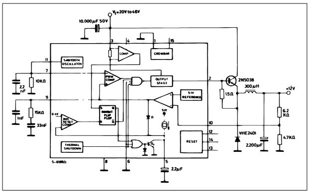
Figure 38 : Programmable Power Supply.
