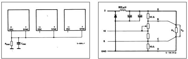
Figure 40 : In Multiple Supplies Several L296s can be Synchronized As Shown.
