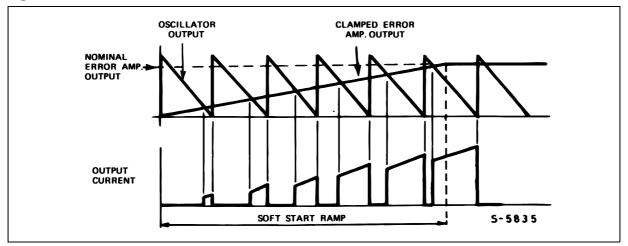
Figure 3 : Current Limiter Waveforms
