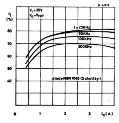
Figure 30 : Efficiency vs. Output Voltage.
