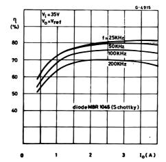
Figure 28 : Efficiency vs. Output Current.
