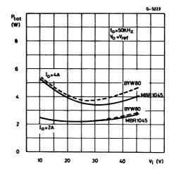
Figure 25 : Power Dissipation (device only) vs. Output Voltage (see fig. 4).
