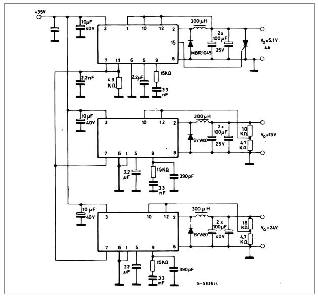
Figure 43: 5.1V/2A Power Supply using External Limiting Current Resistor and Crowbar Protection on the Supply Voltage (L296P only)
