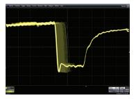
No infrequent glitches and less edge jitter were observed after 30 seconds of persistence on the LeCroy 1, even with WaveStream enabled.
