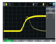
Multiple infrequent glitches and metastable signals were observed after one second of persistence on the 4000 X-Series.
