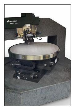
The Keysight Technologies, Inc. 5600LS AFM, already one of the most versatile atomic force microscopy systems on the market (with a fully programmable 200 mm stage that allows complete access over a full 200 mm in X/Y travel), has added yet another highly useful configuration.
