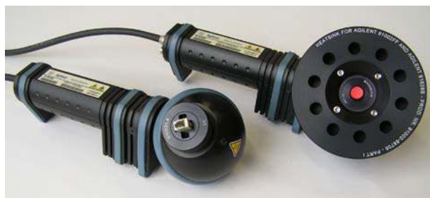
81628B InGaAs head with integrating sphere
