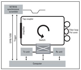
Figure 1. Recirculating loop experiments
