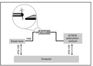
Figure 3. Alignment of polarization maintaining fibers
