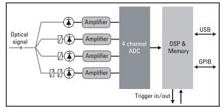
Figure 2. Keysight N7781B polarization analyzer setup
