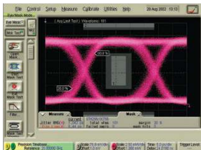
Characteristic optical unfiltered eye measurement (86116C-041).
