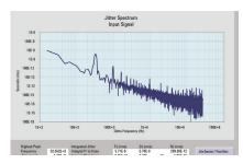
The phase noise plot provides valuable insights into the nature of random jitter. Different noise mechanisms have different profiles.
