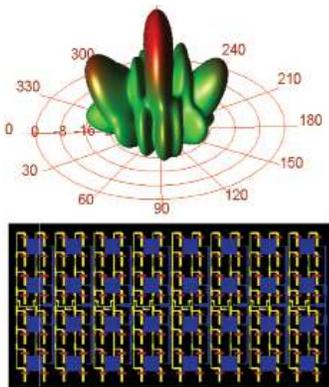
Use Momentum Turbo to quickly analyze large planar phased-array antennas through multi-threaded parallel simulation with optimized NlogN algorithm and adaptive frequency sweep.
