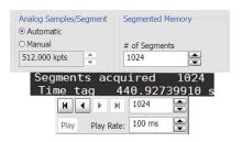
Capture seconds to days of serial protocol. The scope fills memory as each acquisition sees it's trigger condition.
