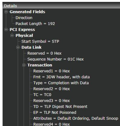
Details window shows hierarchy of physical datalink and transaction layers. Hovering shows additional detail.
