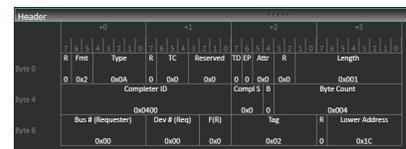
Header window shows packets in a data book format. Hovering at any field reveals additional detail. In this example memory completion packet header is shown.
