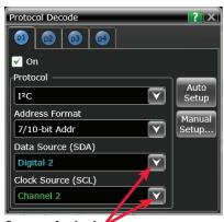
Support for both analog and digital channels
