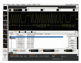
Quickly move between physical and protocol layer information using the time-correlated tracing marker. Display protocol content using embedded decode in the waveform area, Or, see protocol events in a compact listing format. View the decode information in symbols or packets type.
