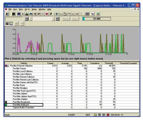
Keysight Protocol Vitals allow you to examine traffic before and after applying filters
