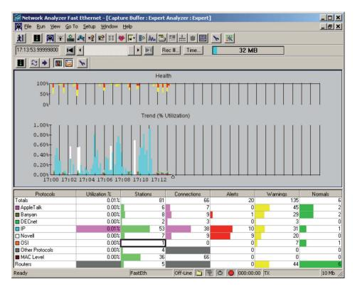
Keysight's Expert Analyzer summarizes network conditions in a simple screen, with drill-down capabilities for major details.
