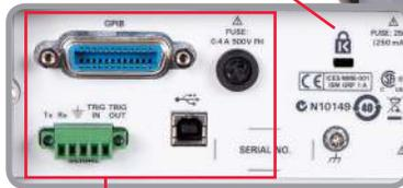
Multiple choices of connectivity and trigger in/out capability for production data analysis
