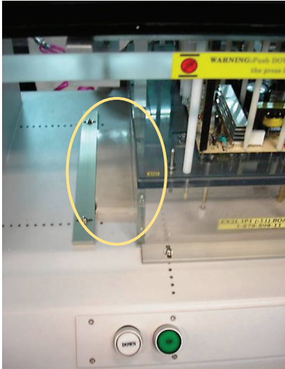
Figure 7. Spacer bar added between bar and fixture.
