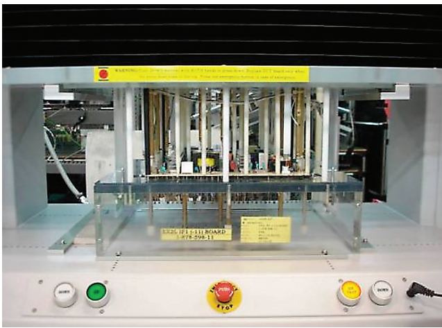
Figure 10. Fixture engaged with 2/3 probe compression.
