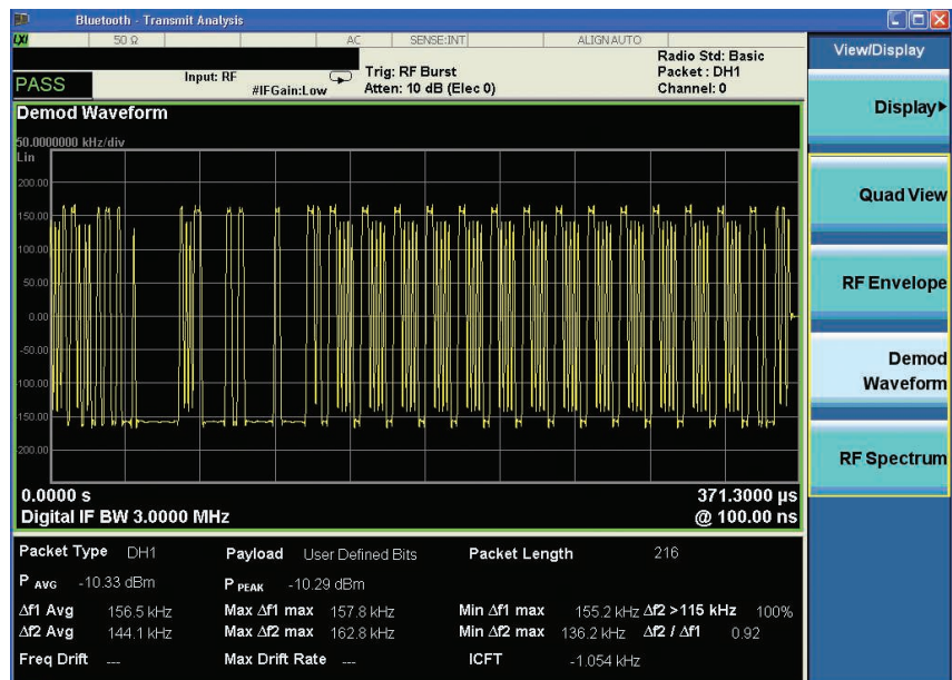
Figure 6. The demodulation waveform shows the modulation characteristics measurement for the Bluetooth basic rate
