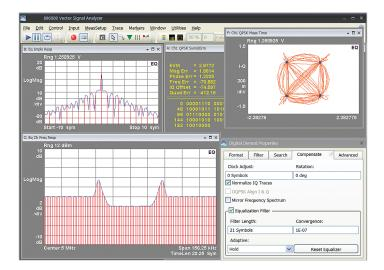
The equalizer channel frequency response is used to evaluate multi-path effects, and its impulse response coeffi cients are available for download. When running the equalizer, the Demod Properties window remains conveniently visible for access to the Run/Hold control during tuning.
