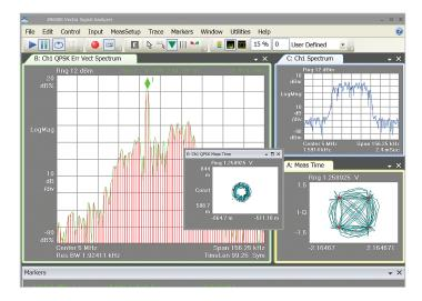
The EVM spectrum measurement shows an interfering signal coupling in from another part of the circuit.
