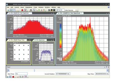
Save a signal and re-analyze it later with the Option AYA tools. Here, the spectrum and constellation appear to be fine. Even the EVM spectrum (trace C) is fine. But the cumulative history display of the EVM spectrum (trace E), which can highlight signal performance over  $\gt500$  hours, detects a transient error.
