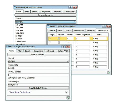
Flexible digital demodulation lets you adjust many important modulation parameters, and customize your own APSK signal analysis
