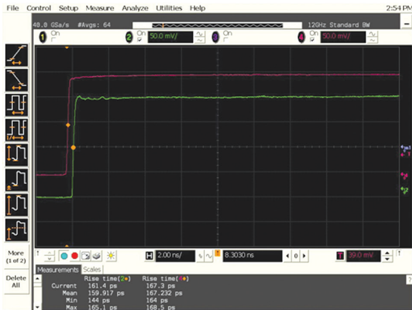
Figure 4 Time domain differential probe response, purple = input of the probe, green = probe output, using Keysight 1169A InfiniiMax probe and DSO81304B 13 GHz oscilloscope
