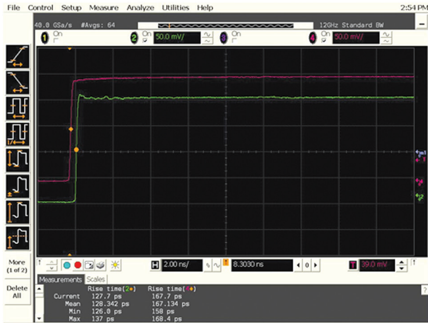
Figure 5 Time domain single-ended probe response, purple = input of the probe, green = probe output, using Keysight 1169A InfiniiMax probe and DSO81304B 13 GHz oscilloscope
