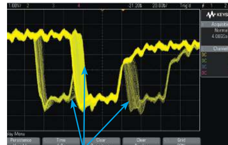
Infrequent glitches and signal jitter captured after 1 second on 3000 X-Series with > 1,000,000 wfms/s
