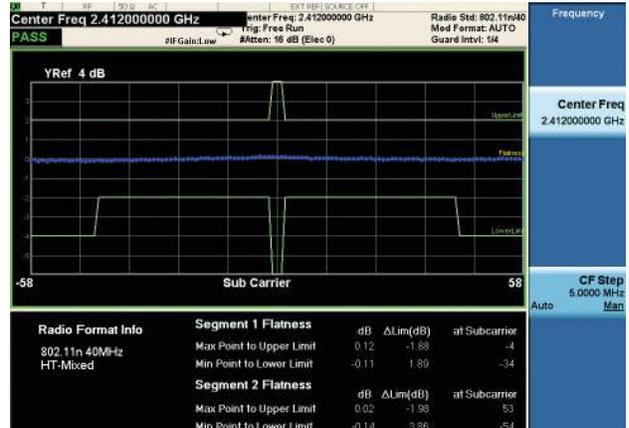
Figure 4. Spectrum flatness of a 40 MHz IEEE 802.11n signal (Greenfield mode).
