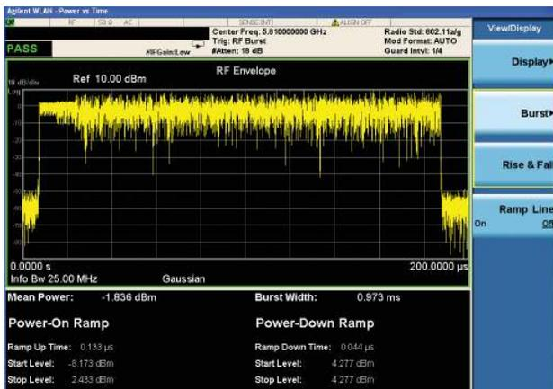
Figure 5. Time-domain view of an 802.11a burst.
