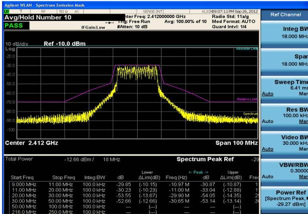
Figure 3. Transmit spectrum mask measurement showing IEEE defined limits.
