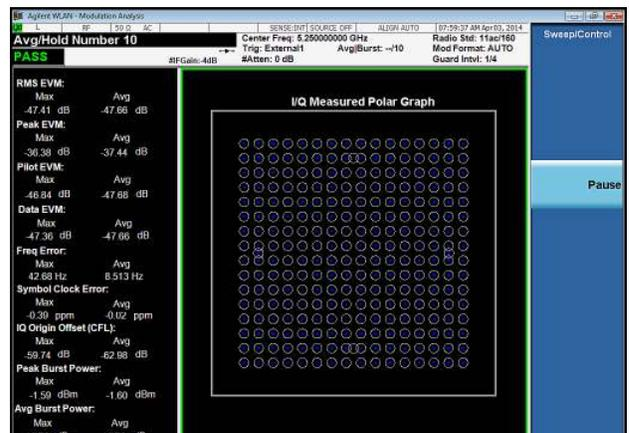
Figure 6. Modulation analysis of a 160 MHz 802.11ac signal with MCS 9 256QAM signal.
