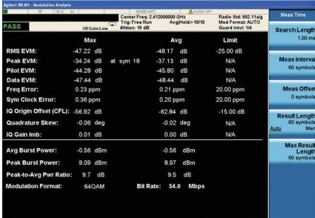
Figure 1. Numerical results summarize modulation accuracy parameters for WLAN signals.
