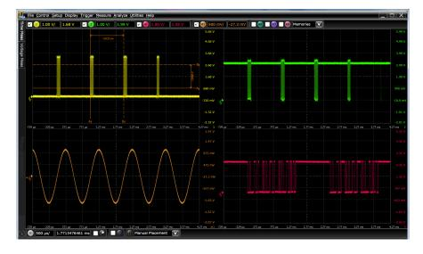
Open up to 8 signals one by one, or use Keysight's composite file to open/save everything in a single mouse click. Composite files include all setup settings, all analog and memory waveforms, and window positioning.
