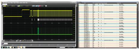
The decode listing window can be displayed simultaneously with the waveform window, configured as an unique window tab, or undocked and moved to any location on your PC monitor including on extended or multi-displays.
