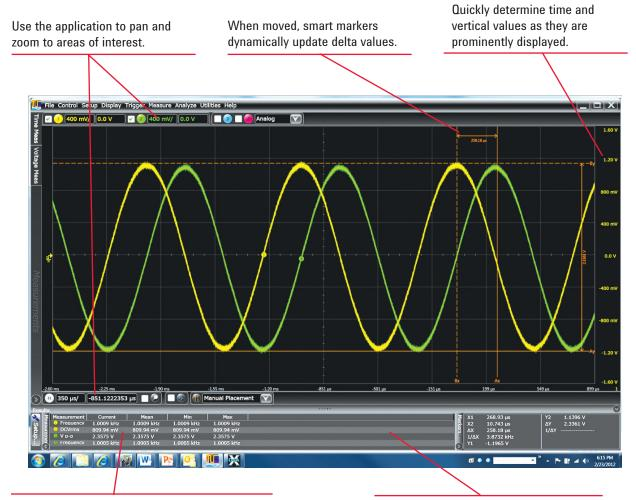
Make quick and precise measurements using drag and drop, or by choosing from any of the 50 built-in automated measurements.
