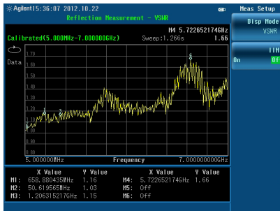
Using the option RM7 for reflection measurements
