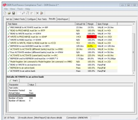
The 16850 Series offers not only memory decode on addr/cmd for up to DDR2/3 1333, but also allows for conformance testing as shown.
