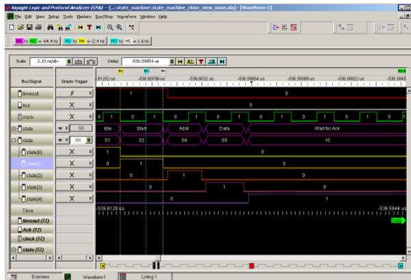
Often it is easy to trigger on a symptom of a problem, like an error flag. In this example, one can look far back in time before the trigger with 2.5 GHz (400 ps) timing to see the timing and functional details of the root cause of failure.
