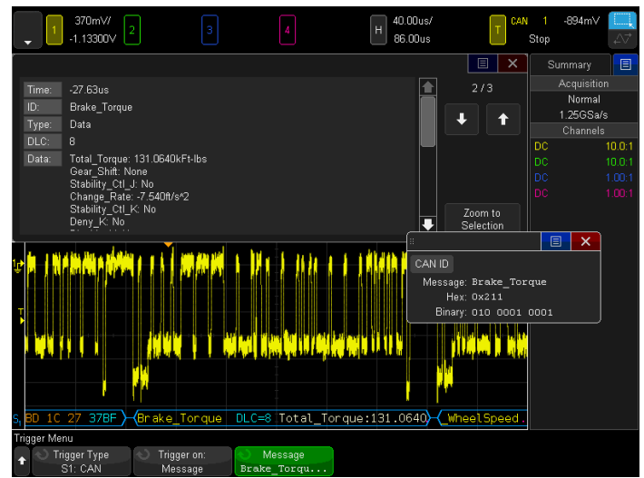
Figure 2a. Symbolically triggering on and decoding the CAN bus.
